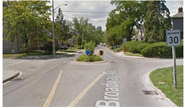
A **mini roundabout** reduces the number of stops on a cycling route in Toronto.
