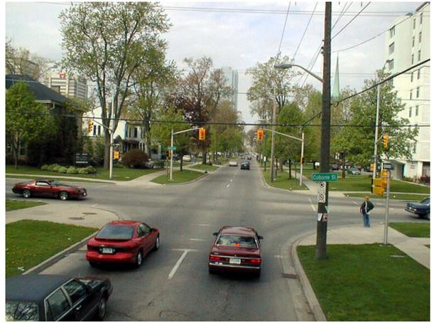
Overhead electricity and communications cables provide easier access but are vulnerable to tree/ice damage and detract from the streetscape's experience.
