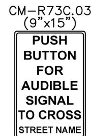
The minimum walk time shall be 10 seconds for crossing with accessible pedestrian signals. Pedestrian clearance time shall be based on the requirements of the latest edition of the [Ohio Manual of Uniform Traffic Control Devices](#).
