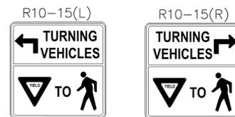
The sign shall be mounted overhead 3’ to the left of the left-most head for the R10-15(L) or 3’ to the right of the right most head for the R10-15(R).
