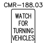
These signs shall be installed on the same pole or pedestal as the corresponding pedestrian signal head.
