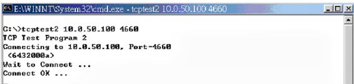
Figure 6.2 TCP test sample program in Visual C
