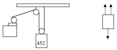
The only tricky part of this is to realize that all of the cords have the same tension, so the free body diagram looks like this and (with tension in the opposite direction from the acceleration).
