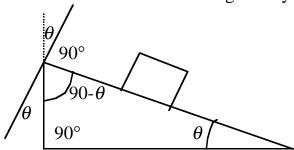
We draw a free body diagram for the case when there is no friction between the object and the surface. Inclined plane problems are usually easier to solve if we chose the "x" axis along the incline. (In general, always chose the direction of acceleration as one of the axes).
