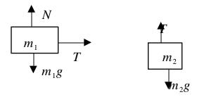
The tensions must be the same and the accelerations must be the same, so for block 1 tension and acceleration are in the same direction.
