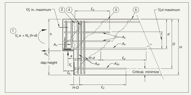
Page 5–77, Figure 5.5.4 (b): Replace figure with the following to delete the dowel bar and vertical plate at the bearing angle:
