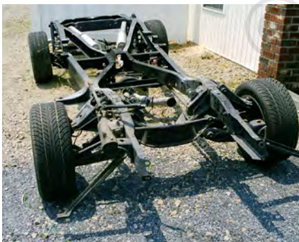
Fig. 3.1: Chassis with suspension and exhaust system
