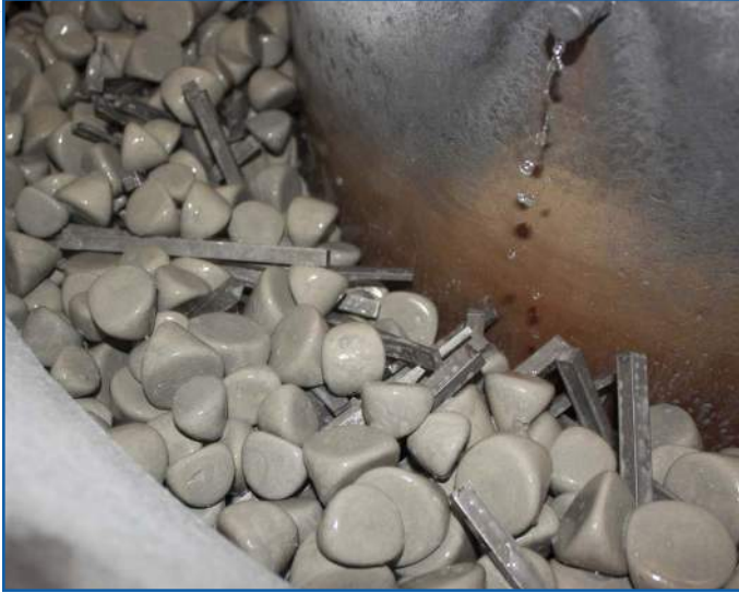
Tumbling removes burrs resulting from machining and black scale resulting from heat treatments.
