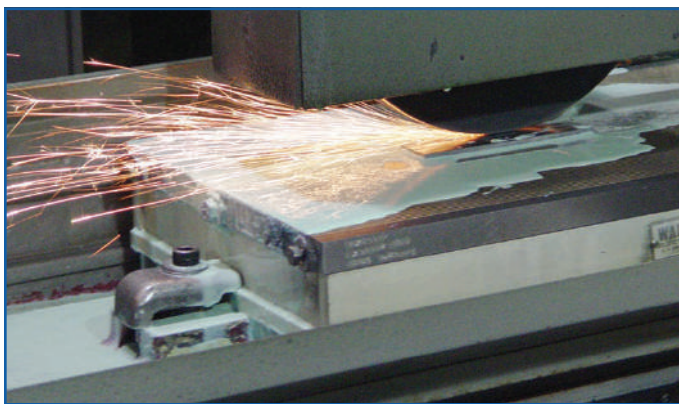
Grinding creates carrier lines and sprigs caused by the combustion of the constituent elements which can help identify the chemical composition of a particular piece of metal.
