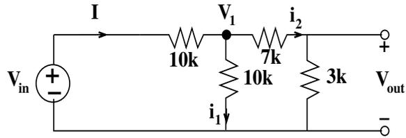
(c) (3 pts) What is  $V_1$  in terms of  $V_{in}$ ?  $V_{in}/3$
