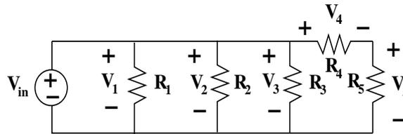
(f) (2 pts) What is  $V_1 + V_2 + V_3$  in terms of  $V_{in}$ ?  $3V_{in}$
