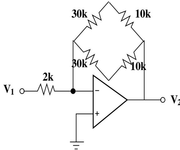
$$V_2 = -10V_1$$
