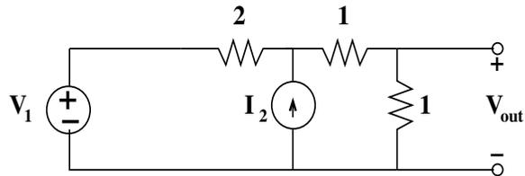
(a) (6 pts) What is  $V_{out}$  in terms of  $V_1$  and  $I_2$ ?  $V_{out} = \frac{V_1}{4} + \frac{I_2}{2}$
