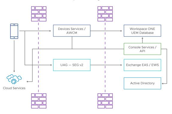
Figure 18: BB Clothiers' network architecture diagram.
