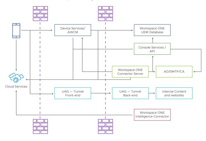
Figure 15: TRC network architecture diagram.
