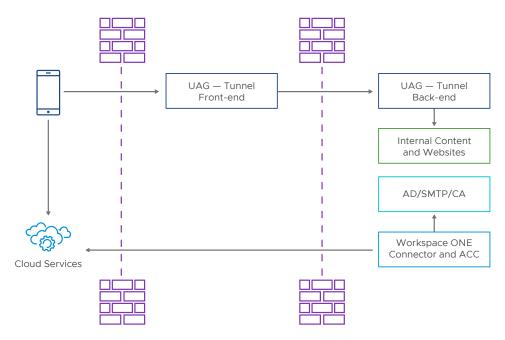
Figure 12: Flancrest's network architecture diagram.
