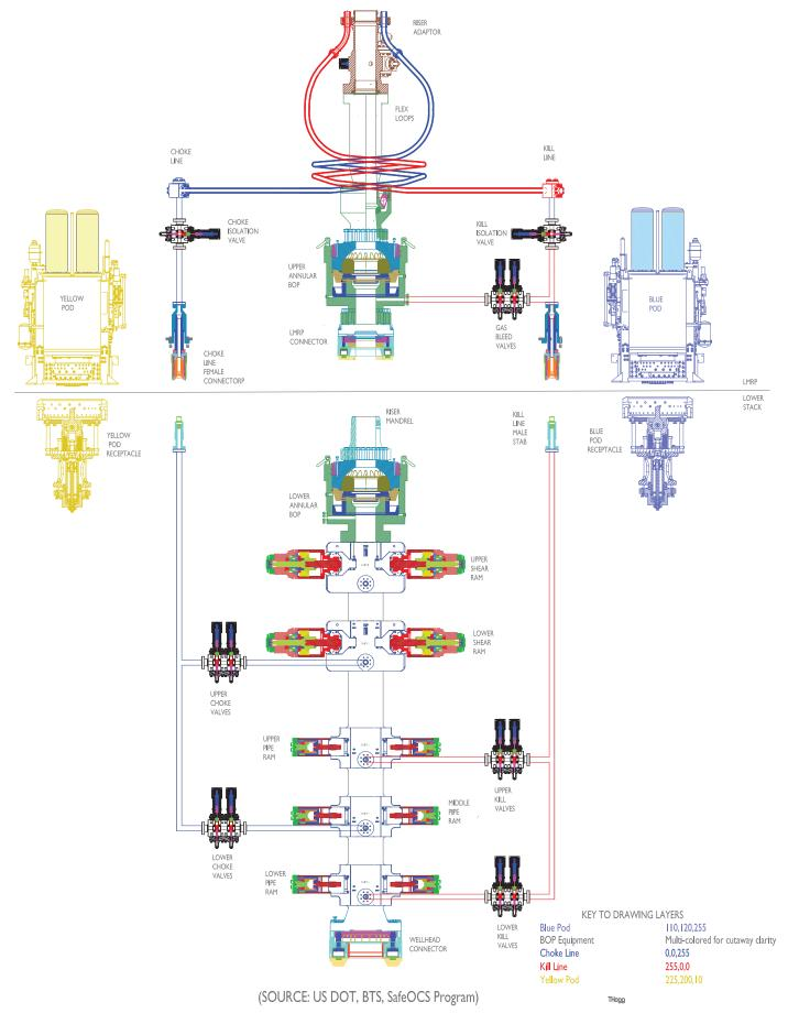
Figure F. Example Schematic for Surface BOP Stack Control System
