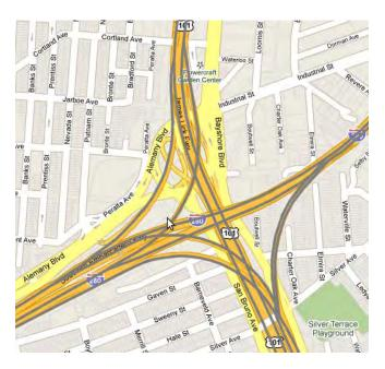
(b) Simplified representation (in gray) of the interchange for traffic estimation algorithms overlayed on a Google map of the area. Although not pictured, the estimation algorithms are aware of the incoming and outgoing ramps, allowing them to account for incoming and exiting traffic while not worrying about modeling the ramp traffic conditions explicitly.
