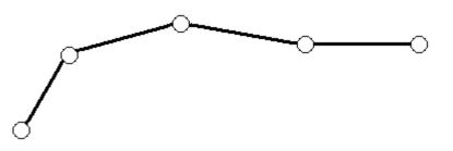
Figure 2.1. A link is an ordered series of two or more points that represent the geometry of a road segment, geometrically known as a "linestring".
