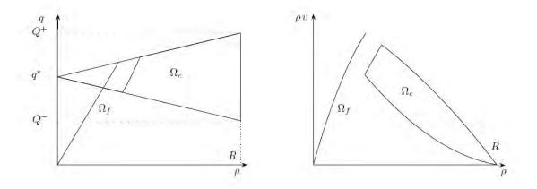
Figure 2.1. Colombo phase transition model. Left: Fundamental diagram in state space coordinates  $(\rho, q)$ . Right: Fundamental diagram in density flux coordinates  $(\rho, \rho v)$ .
