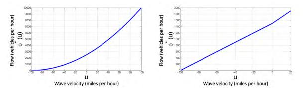
Figure 3.1. Illustration of the convex transforms associated with the Greenshields and trapezoidal Hamiltonians.
