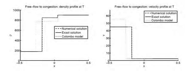
Figure 5.2. Exact solution (continuous line), computed solution (dashed line), and solution to the Colombo model (dotted line) for density (left) and speed (right). Between the two initial states appears a state  $u_m = (847.4, -0.24)$  which corresponds to the intersection of the lower bound of the diagram in congestion with the 2-Lax curve going through  $u_r$ . In this graph T = 1 and  $\Delta x = 0.0013$ .
