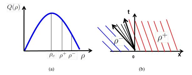
Figure 3.5. Riemann problem solved by a rarefaction wave moving back. (a) initial data; (b) evolution of the characteristic curves.
