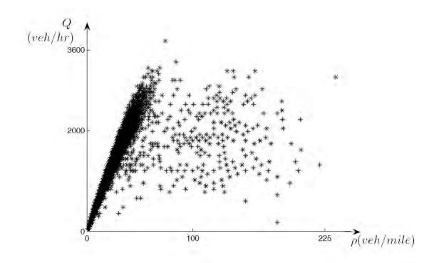
Figure 3.1. Fundamental diagram in density flux coordinates from a street in Rome. In congestion (high densities) the flux is multi-valued. Count *C* and velocity v were recorded every minute during one week. Flux *Q* was computed from the count. Density  $\rho$  was computed from flux and velocity according to the expression  $Q = \rho v$  (see [75] for an extensive analysis of this dataset).
