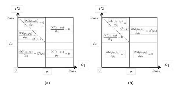
Figure 4.2. Summary of the computation of (a)  $\frac{\partial G(\rho_1,\rho_2)}{\partial \rho_1}$ ; (b)  $\frac{\partial G(\rho_1,\rho_2)}{\partial \rho_2}$ . Note that the line connecting  $(\rho_c, \rho_c)$  and  $(0, \rho_{\max})$  may have different shapes depending on the flux function  $Q(\cdot)$ , and represents the set for which  $G(\cdot, \cdot)$  is not differentiable.
