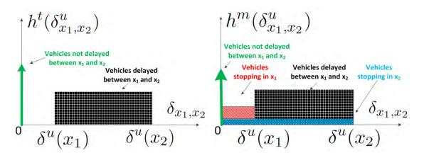
Figure 3.3. (Left) Probability distribution of the total delay between  $x_1$  and  $x_2$  in the undersaturated regime. (Right) Probability distribution of the measured delay between  $x_1$  and  $x_2$  in the undersaturated regime. Vehicles are assumed to be sampled uniformly in time.
