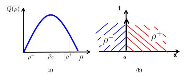
Figure 3.9. Riemann problem solved by a big stationary shock. (a) initial data; (b) evolution of the characteristic curves.
