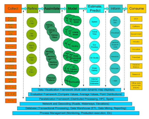
Figure 1.4. Final Mobile Millennium expanded data flow diagram
