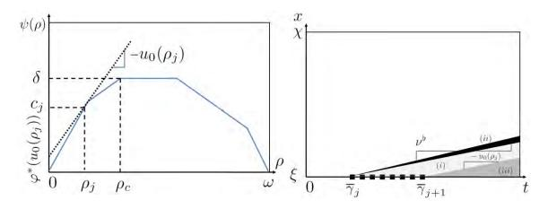
Figure 5.2. Construction of the solution associated with an affine upstream boundary condition.
