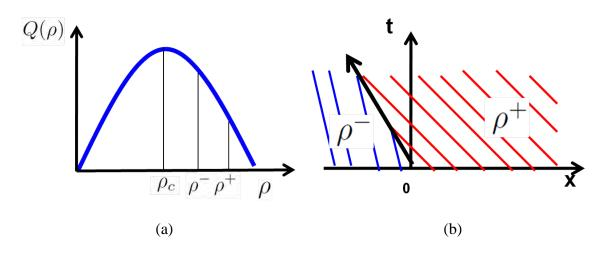
Figure 3.4. Riemann problem solved by a small shock wave moving back. (a) initial data; (b) evolution of the characteristic curves.
