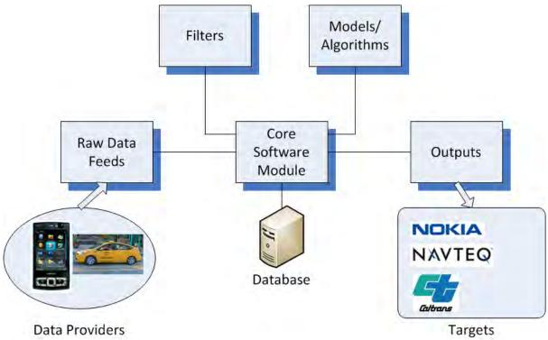
Figure 3.3. Mobile Millennium system database-centric architecture.
