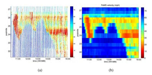
Figure 2.1. I-880N experiment data. (a) Vehicle GPS logs stored locally on the phone. (b) PeMS velocity contour plot. Color denotes speed in mph. *x*-axis: time of day. *y*-axis: postmile.
