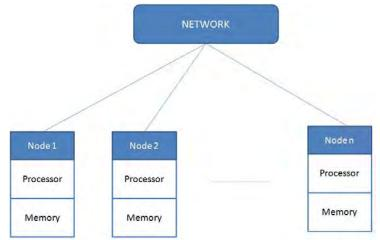
Figure 2.1. Structure of a HPC Cluster
