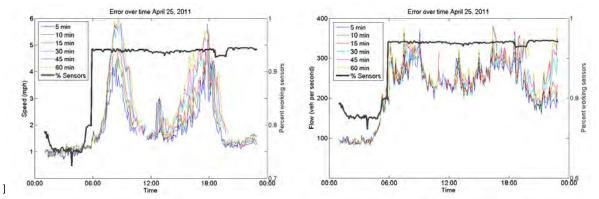
thicker solid line indicates the percentage of "healthy" sensors at the corresponding moment in time (and corresponds to the right y-axis on the plot).
