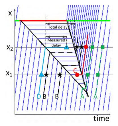
Figure 3.2. Classification of the trajectories depending on the stopping location. We consider vehicles traveling between the two measurement points  $x_1$  and  $x_2$ , sampled uniformly in time.
