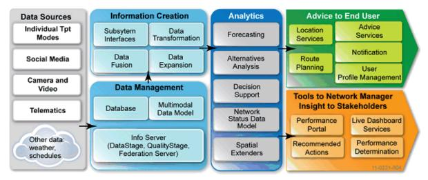
Figure 1.2. Data from various sources are consumed by information creation and data analytics tools prior to becoming custom output for Smarter Traveler end users.
