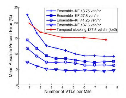
Figure 5.4. Tradeoffs between number of virtual trip lines per mile and the travel time error for different values of the number of equipped vehicles sending measurements per hour.
