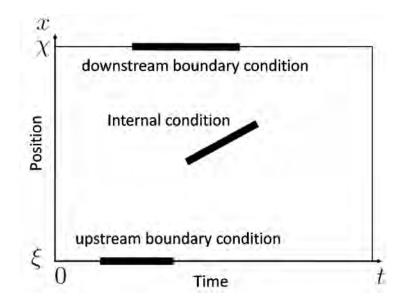
Figure 1.2. Illustration of the domains of the possible value conditions used to construct the solution of the Moskowitz HJ PDE.
