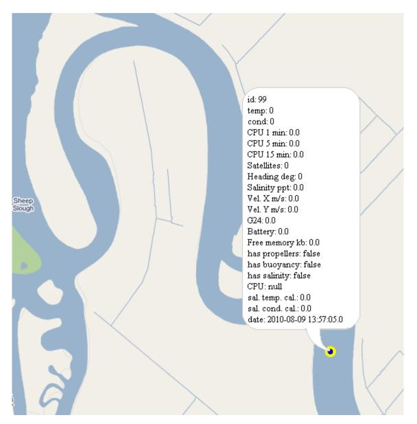
Figure 4.4. Location and status of a Drifter robot shown in FLO\_VIZ.
