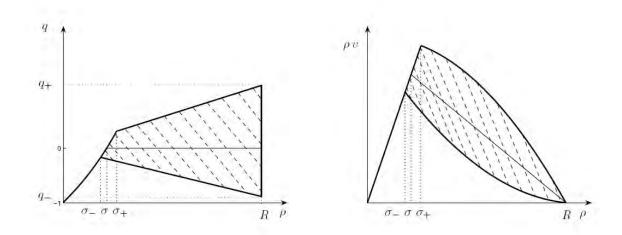
Figure 3.2. Newell-Daganzo standard flux function. Left: Fundamental diagram in state space coordinates. Right: Fundamental diagram in flux-density coordinates. The standard state is the usual triangular diagram. The congestion phase is two-dimensional (striped domain).
