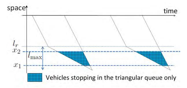
Figure A.2. Case 2: Some vehicles stop in the triangular queue. The others do not experience delay.
