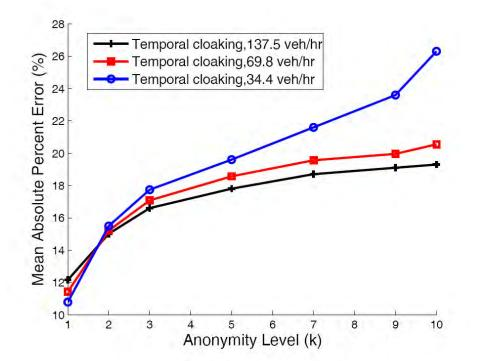
Figure 5.2. Travel Time Accuracy versus Anonymity Level using 10 VTLs/mile.
