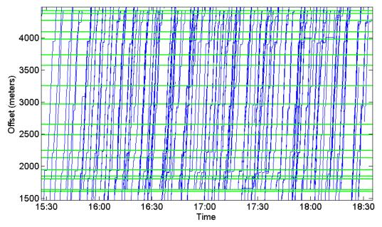
Figure 1.3. Vehicle trajectories from the *Mobile Millennium* evaluation experiment on San Pablo Avenue in Berkeley, Albany and El Cerrito, California. The high-frequency GPS data in this figure is represented as distance (meters) from an arbitrary start point upstream of the experiment location. The horizontal lines represent the locations of the traffic signals along the route.
