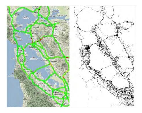
Figure 5.1. Best viewed in color. Velocity estimates on the Bay Area highway network. Right: Cumulated probe speed measurements collected on July 29<sup>th</sup> by the *Mobile Millennium* system. Left: Velocity estimates on July 29<sup>th</sup> at 9 pm; most of the network is in free flow, active bottlenecks correspond to red spots.
