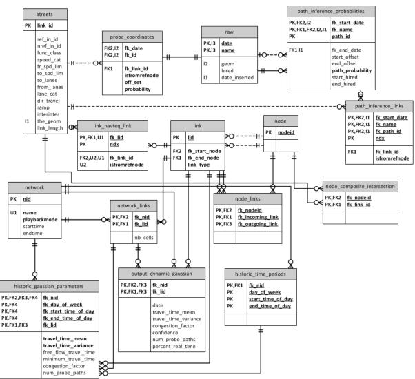
Figure 3.4. An illustration of the relationship between the core tables and a few auxiliary modules of the *Mobile Millennium* database. The symbols between tables represent the relationship between data structures (such as one-to-one, many-to-one, etc.).
