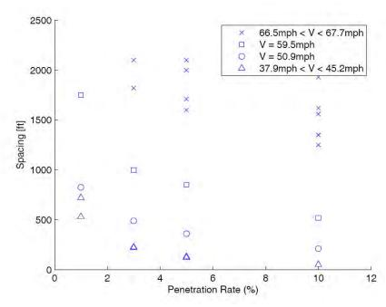
Figure 4.2. Minimum Spacing Constraints for Straight Highway Section.
