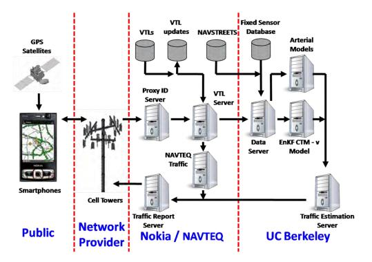
Figure 1.1. Mobile Millennium System Architecture (Nokia and Berkeley)
