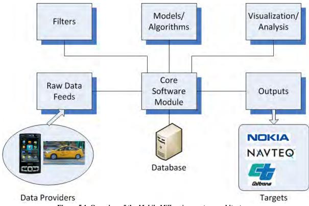
Figure 5.1. Overview of the Mobile Millennium system architecture.
