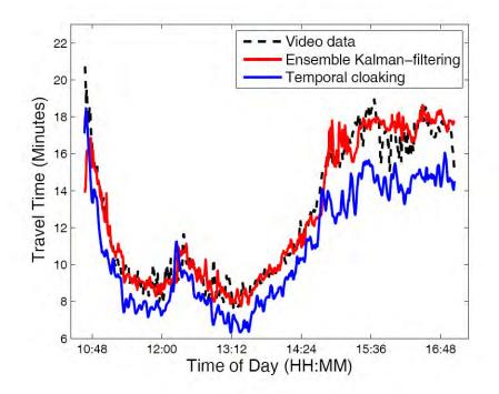
Figure 5.5. Comparison between mean travel time obtained from video data, mean travel time obtained from temporal cloaking, and mean travel time obtained from the accuracy centric architecture.
