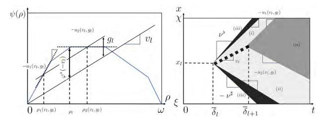
Figure 5.4. Construction of the solution associated with an affine internal condition.
