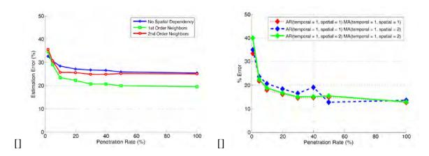
Figure 1.5. Average one-step forecast error vs. penetration rate for all VTL pairs in the **Paramics dataset**. (a) Logistic Regression Forecast Classification Error. (b) STARMA Travel Time Forecast Error.
