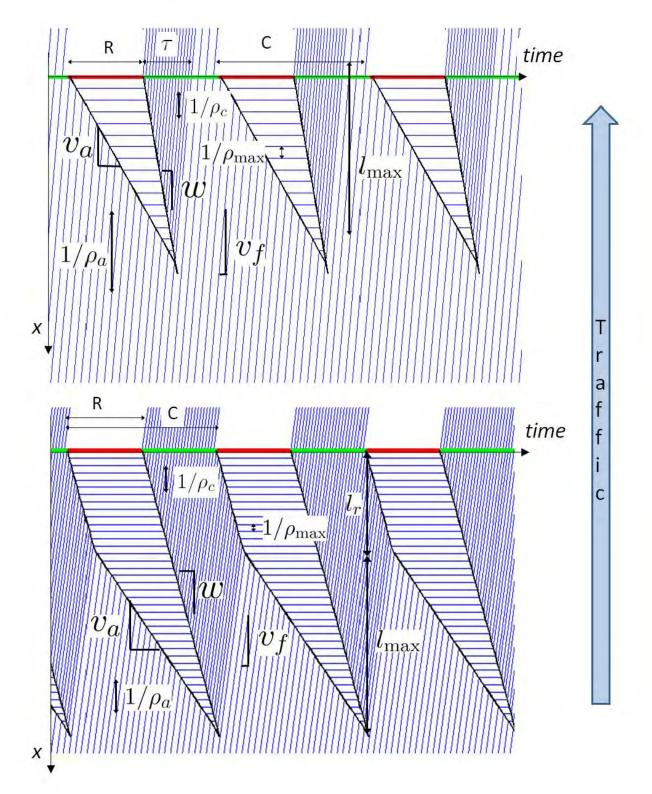
Figure 1.2. Space time diagram of vehicle trajectories with uniform arrivals under an undersaturated traffic regime (top) and a congested traffic regime (bottom).
