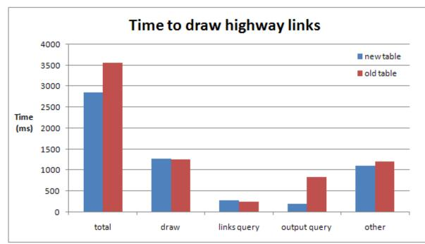
Figure 3.5. This graph shows how a change to the highway model output table improved the speed of VIZ.
