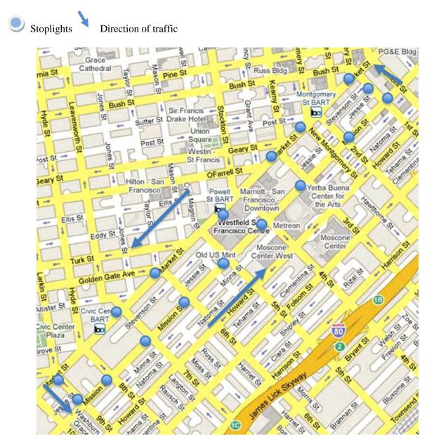
Figure 2.8. Map of the Mission-Market left turn loop utilized for highway/arterial model test 2. Dots indicate traffic signals; arrows indicate the direction of traffic.
