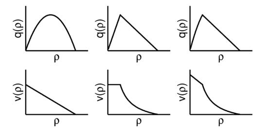
Figure 1.1. Fundamental diagrams (top row) and velocity functions (bottom row) for Greenshields (left), Daganzo-Newell (center), and Smulders (right).
