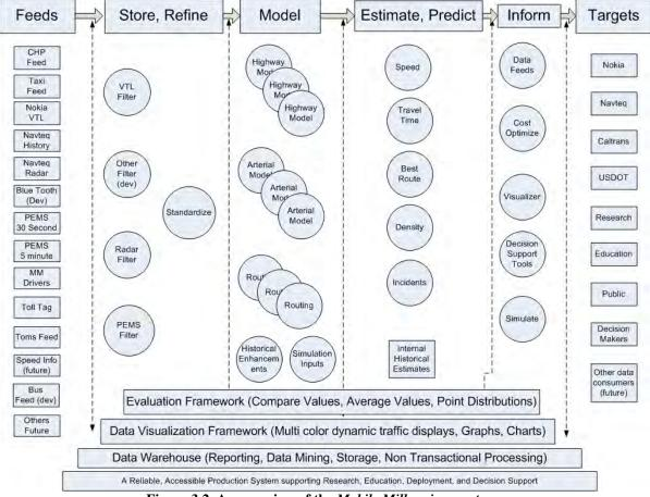
Figure 3.2. An overview of the Mobile Millennium system.
