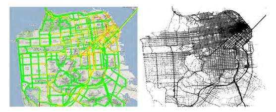
Figure 5.2. Best viewed in color. Travel-time estimates on the San Francisco arterial network. Right: Cumulated probe location measurements collected on July 29<sup>th</sup> by the *Mobile Millennium* system. Left: Travel-time estimates on July 29<sup>th</sup> at 8 pm; green links correspond to free flow travel-times and red spots correspond to congestion.
