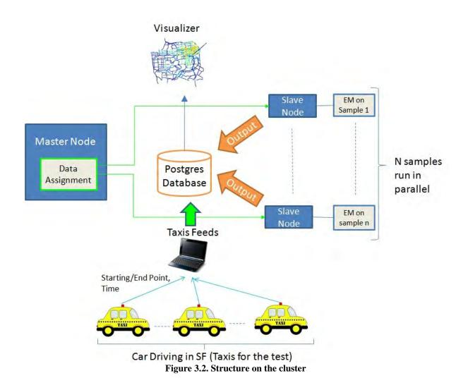
The advantages of using the cluster for the path inference project are that we can run simultaneously an analysis on several samples. The tasks are split among the available nodes and this would reduce the processing time by a factor N (corresponding to the number of slaves available). The structure of the EM algorithm fits well to a deployment on a cluster since each EM task is independent.
