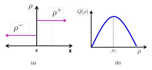
Figure 3.1. (a) Initial data for the Riemann problem; (b) quadratic flux function.
