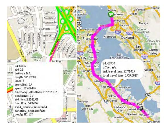
Figure 5.5. Example of map attributes and live trafic data accessible through the Mobile Millennium visualization tool.
