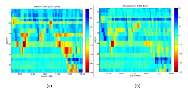
Figure 2.4. PeMS and EnKF CTM-v comparison. Color denotes speed difference between PeMS and EnKF CTM-v with (a) 10 VTLs and (b) 40 VTLs, in mph. Color denotes speed in mph. *x*-axis: time of day. *y*-axis: postmile.
