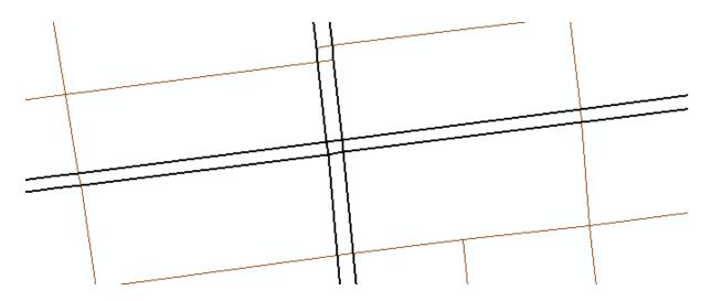
(a) Highway representations of the I280, highway 101 interchange in San Francisco, CA Navteq representation of the intersection. Note that the four small links forming a square in the middle are all approximately 10 meters long each and just represent the distance from one side of the intersection to the other
