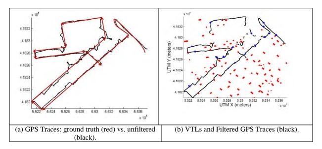
Figure 5.1. In the right figure, red colored lines denote VTLs placed in downtown while blue lines denote detected VTL crossings.
