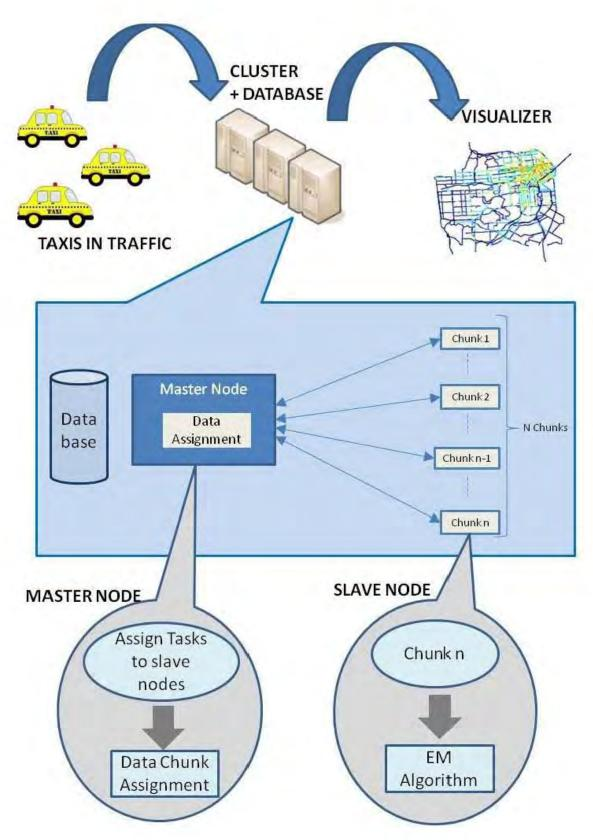
Figure 3.1. Structure of the Path Inference Project
