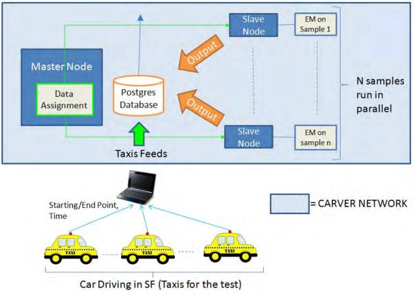
Figure 3.4. Structure of the Path Inference Project on NERSC
