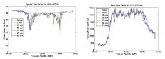
Figure 5.3. Speed and Flow values for VDS 400038. Each line represents a different prediction level.
