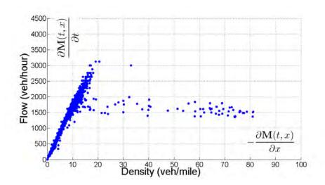
Figure 1.1. Illustration of the flow-density relationship.
