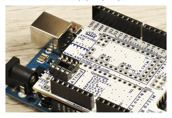
Now it is time to place ATtiny85 on socket. Make sure that pin 1 of the ATtiny85 will be placed properly on ArduShield. Place Attiny85 on ArduSHIELD, and press down gently ATtiny85 up to the point where it stops.
