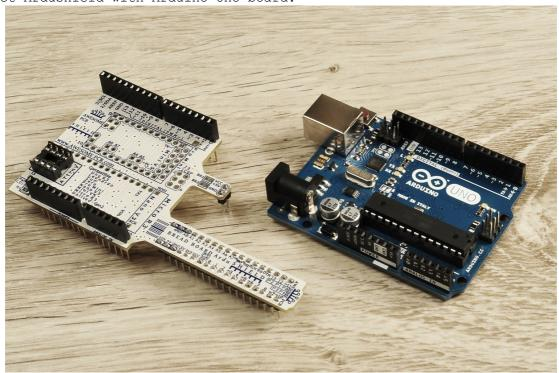
Put the ArduShield on the Arduino Uno and press down gently up to the point where it stops.
