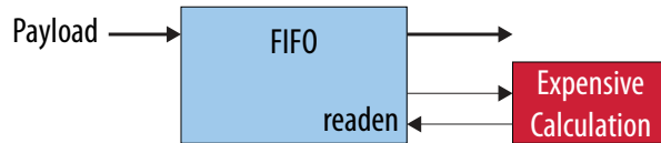
Figure 49. Restructuring a Design with an Expensive Loop
