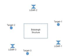
Figure 6 – Layout of the scan and target control point around bobsleigh structure.
