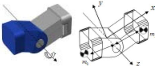
Fig. 5 Rotary joint module with joint axis perpendicular to link.
