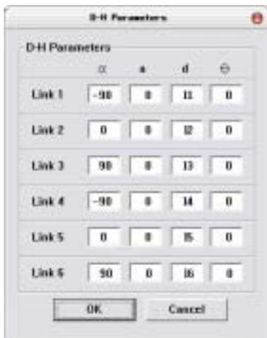
Fig. 11 D-H Parameters from modeling.
