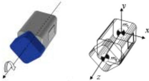
Fig. 4 Revolute joint module with axis coincident with link.
