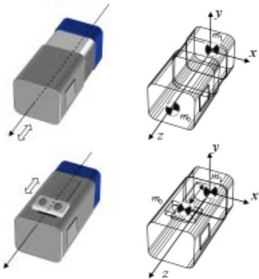
Fig. 6 Prismatic joint module.
