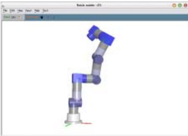
Fig. 10 Geometrical model of a 6 DOF manipulator.
