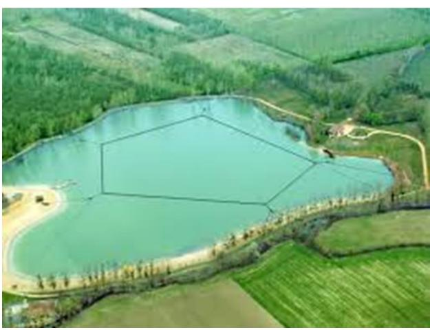
A cable water park includes a lake or river being surrounded by masts which hold an overhead cable. The cable rotates in counter clockwise direction around the lake or straight across the river and has number of carriers. The skiers get pulled by ropes attached to these carriers.
