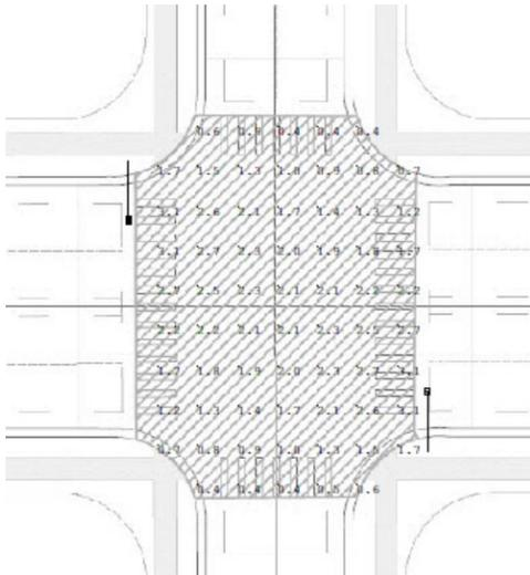
Figure 4: 5' x 5' Grid at Crosswalk for Horizontal Illuminance
