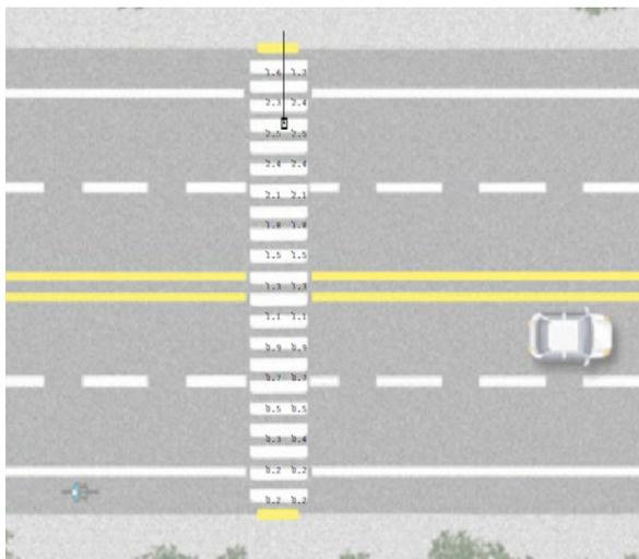
Figure 5: Vertical Illuminance measuring Grid at Mid-block Crosswalk
