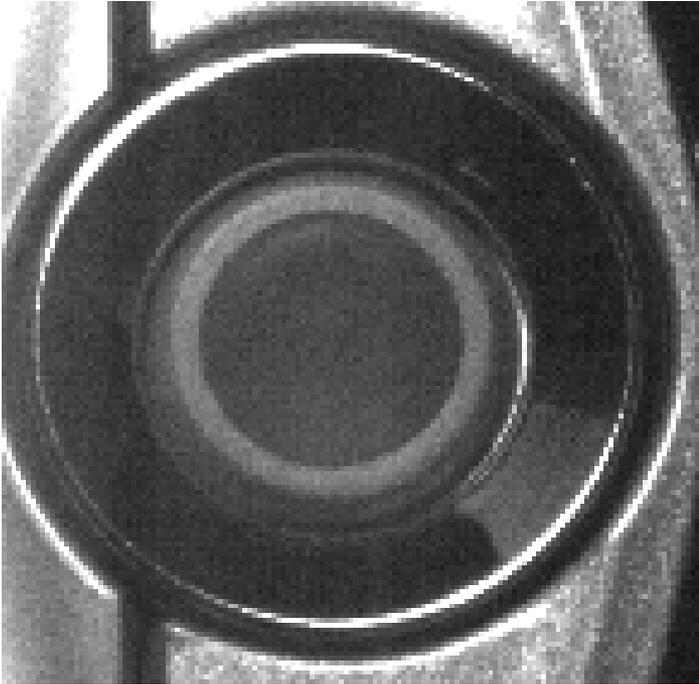
High Gain used to compensate for low light. Bright image, but noise is apparent
