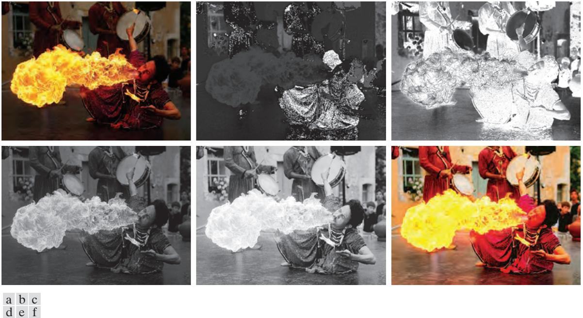
**FIGURE 7.17** (a) RGB image. (b) Hue image. (c) Saturation image. (d) Intensity image. All three images were obtained using function `rgb2hsi`. (e) Histogram-equalized intensity image. (f) RGB image obtained using function `hsi2rgb`. (Original image credit: Luc Viatour, <https://lucnix.be/>.)
