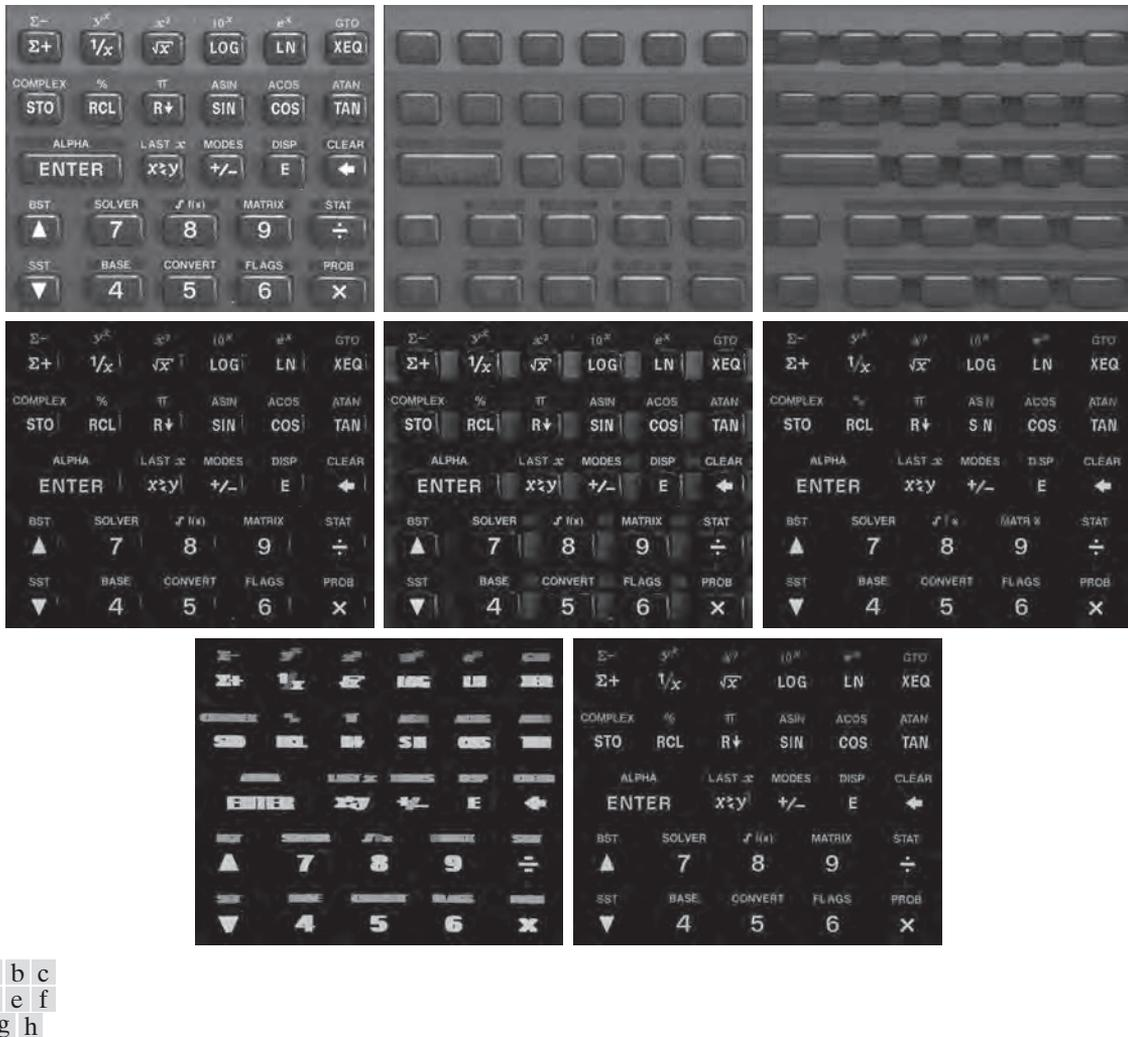
**FIGURE 10.29** An application of grayscale reconstruction. (a) Original image. (b) Opening-by-reconstruction. (c) Opening. (d) Tophat-by-reconstruction. (e) Tophat. (f) Opening-by-reconstruction of (d) using a horizontal line. (g) Dilation of (f) using a horizontal line. (h) Final reconstruction result.
