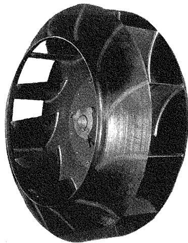
FIGURE 7.25 Centrifugal fan wheel with 12 radial-tip blades, diameter ratio of 0.70. Blades are spaced far enough apart to prevent material buildup. Welded of abrasion-resistant steel. (Courtesy of Chicago Blower Corporation, Glendale Heights, Ill.)
