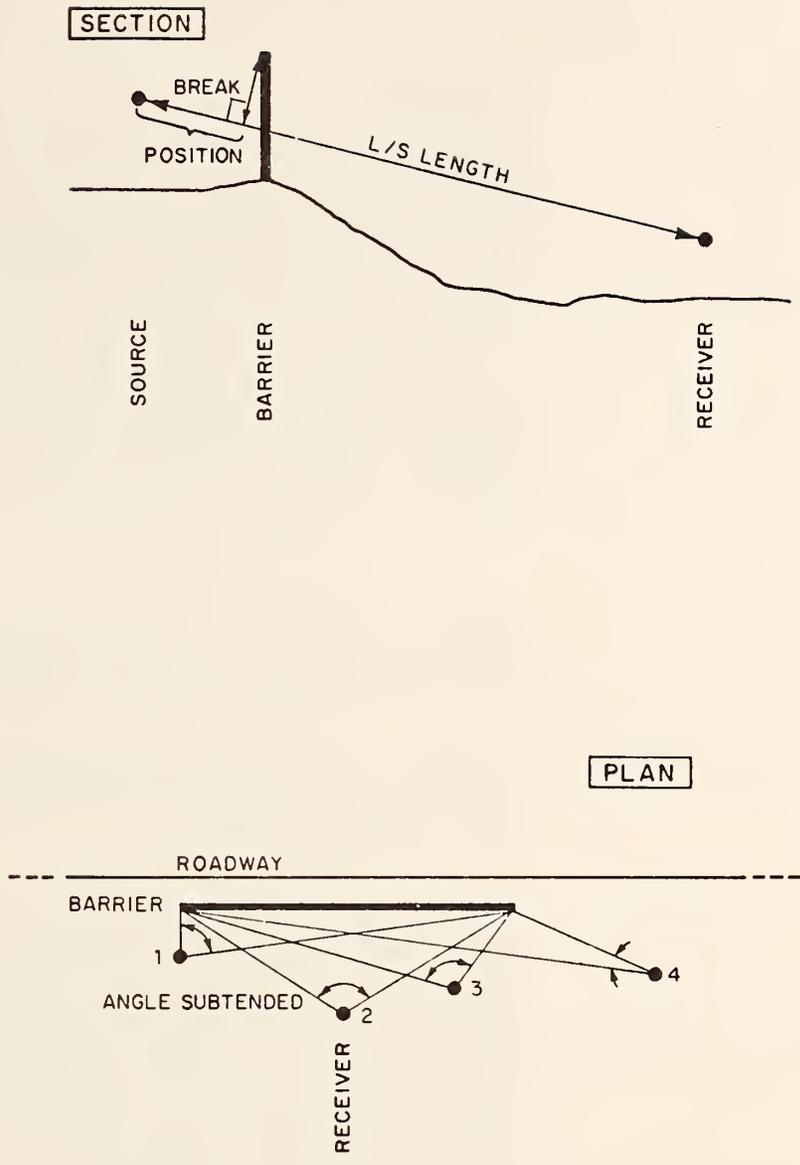
FIGURE 4-10 Illustration of Barrier Parameters.
