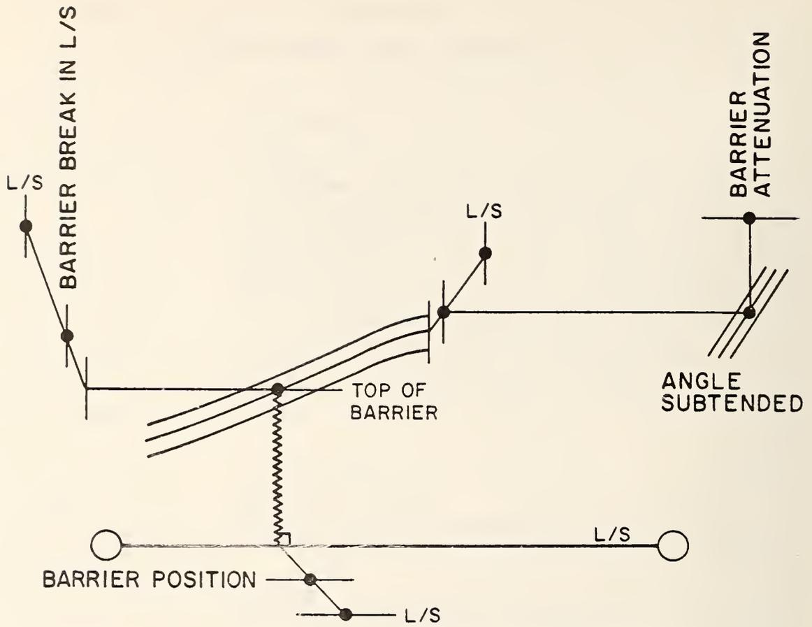
FIGURE 4-12 Overview of Barrier Nomograph.
