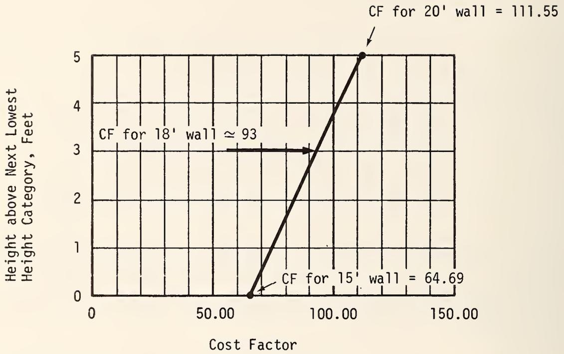
FIGURE 4-36 Use of Grid to Determine Cost Factor.
