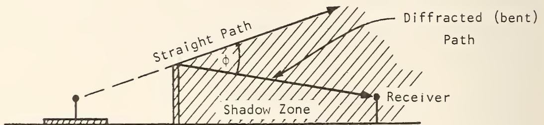
FIGURE 2-2 Barrier Diffraction.
