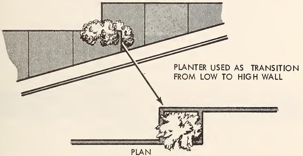
FIGURE 3-21. CONNECTING DIFFERENT HEIGHT WALLS TO VARY VISUAL FORM
