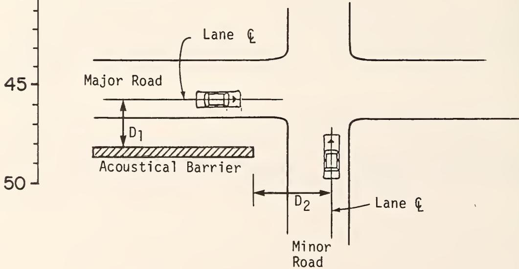
FIGURE 4-8 Safety Factors for Intersecting Roads.
