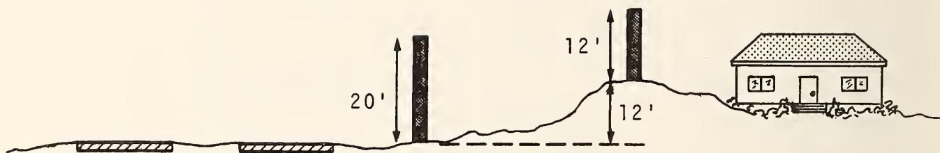
FIGURE 3-4 Use of Elevated Terrain to Achieve Greater Attenuation with Lower Walls.
