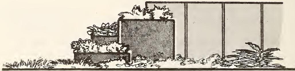
FIGURE 3-25. USE OF PLANTER TO TERMINATE WALL
