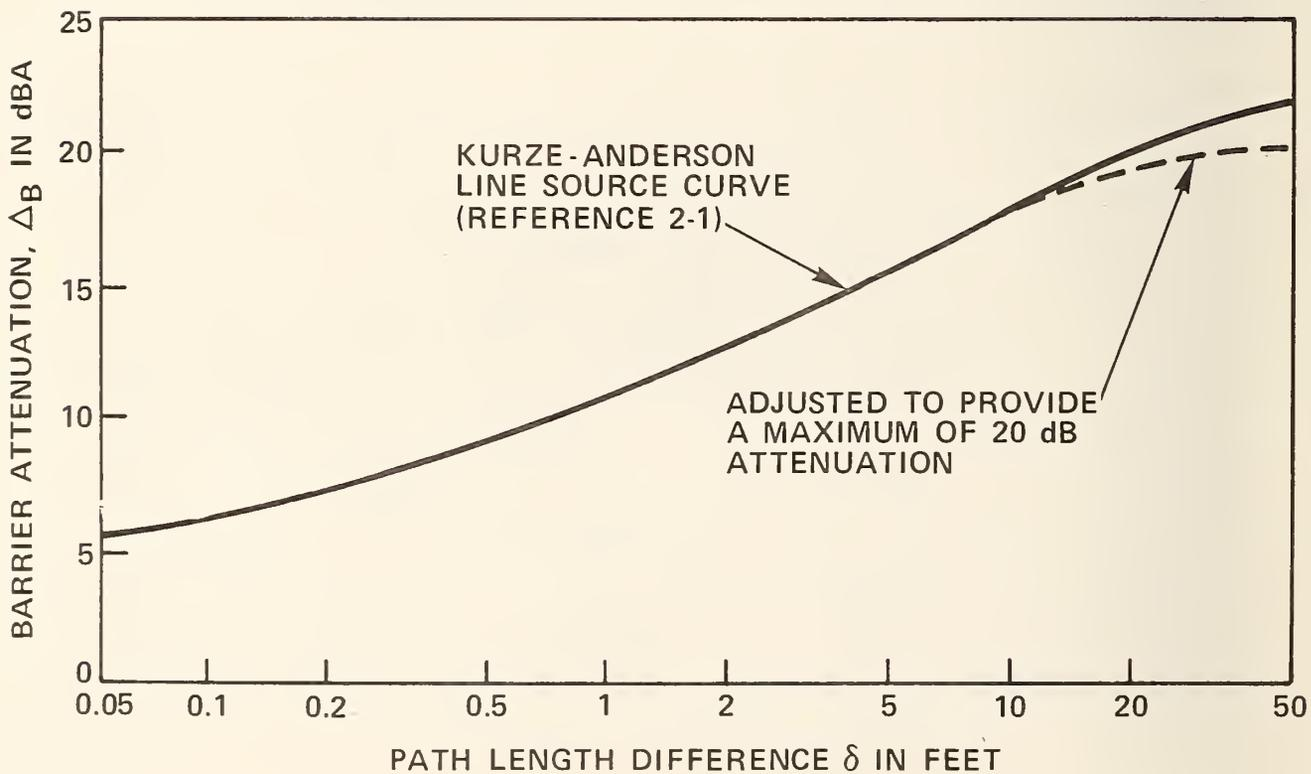
FIGURE 2-4 BARRIER ATTENUATION FOR A LINE OF INCOHERENT POINT SOURCES.
