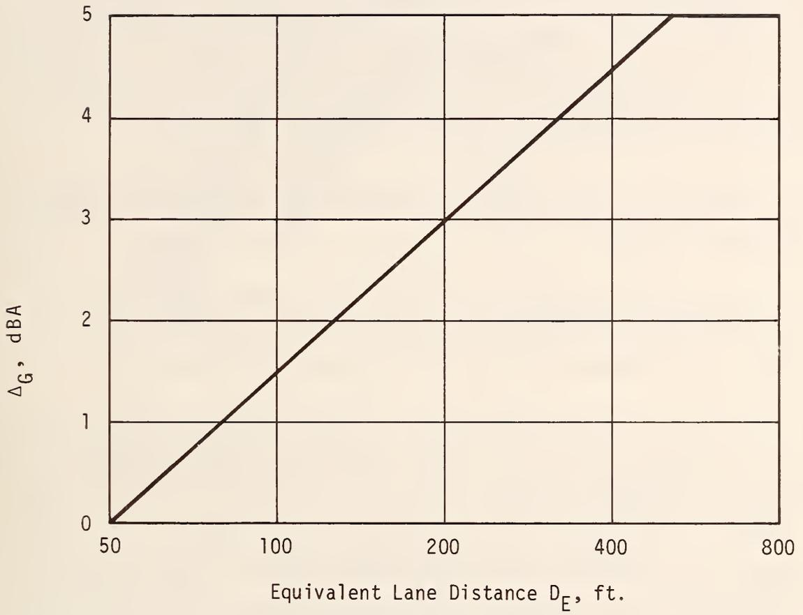
FIGURE 4-3 Ground Effect Attenuation.
