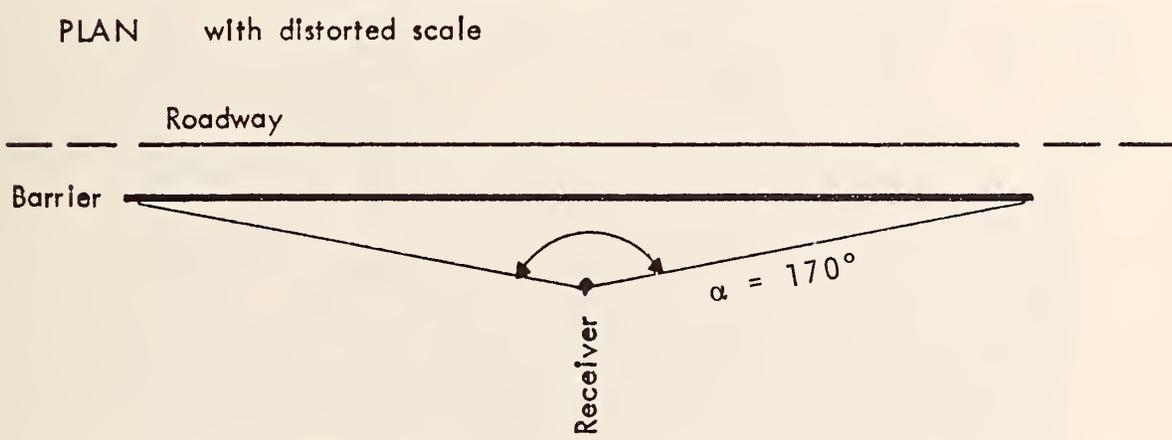
FIGURE 4-14 Barrier Attenuation Example.
