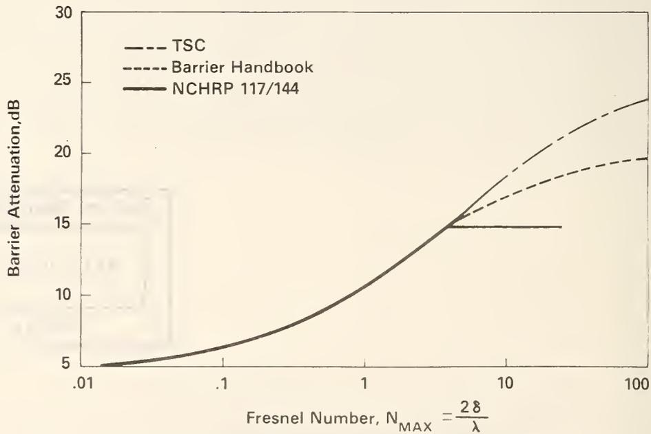
Figure 1. Comparison of approved barrier attenuation curves for incoherent line source.
