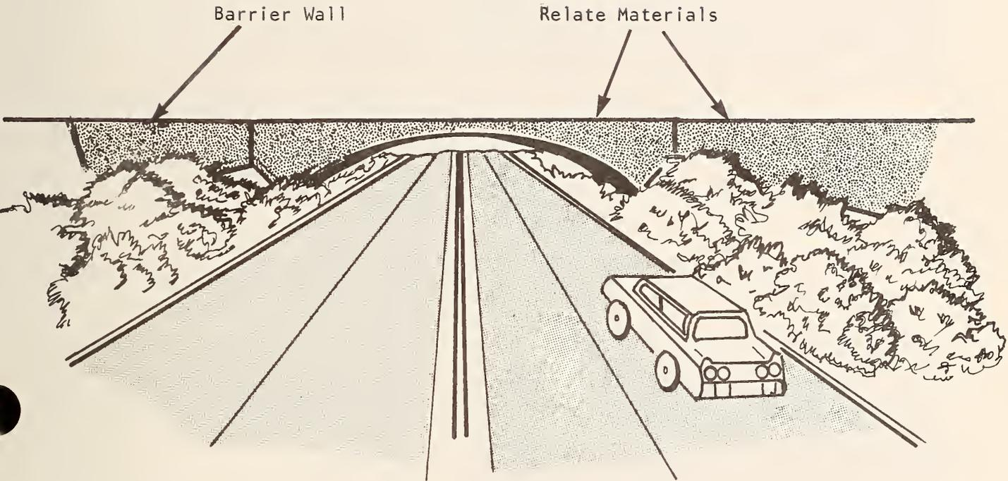
FIGURE 3-18. RELATING BARRIER DESIGN TO OTHER HIGHWAY ELEMENTS
