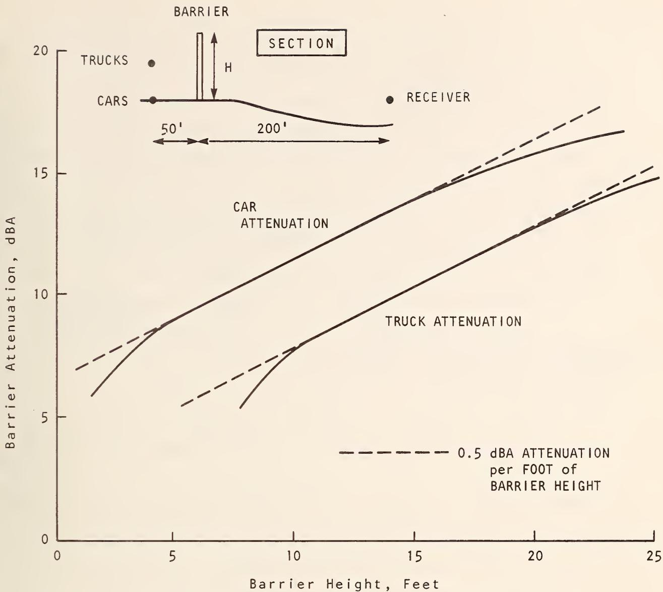
FIGURE 3-3 Barrier Attenuation as a Function of Barrier Height.
