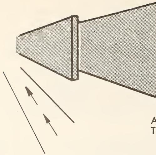
AVOID END WALLS EXPOSED TO FLOW OF TRAFFIC
