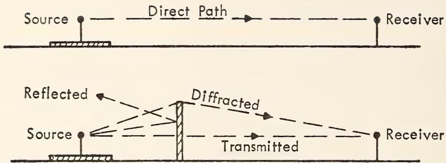
FIGURE 2-1 Alteration of Noise Paths by a Barrier.
