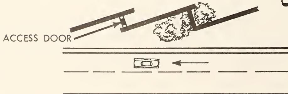
FIGURE 3-13. PROVIDING ACCESS FOR BARRIER MAINTENANCE
