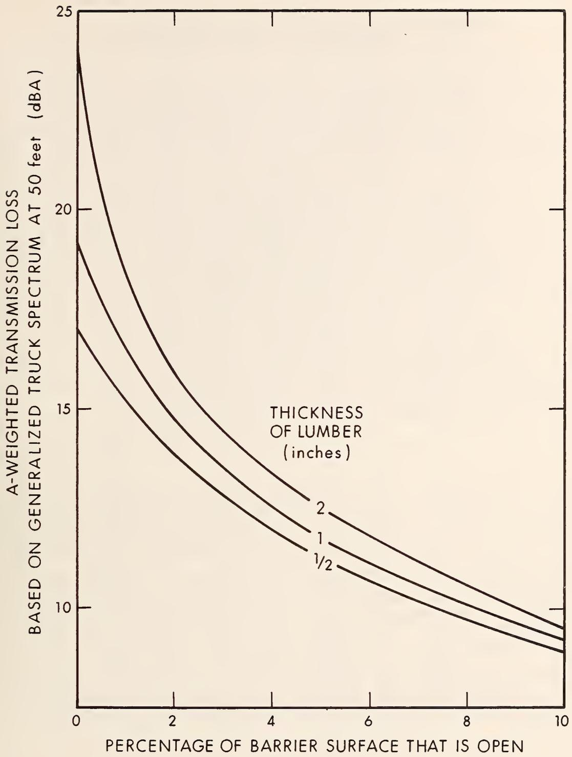
FIGURE 4-28 Effect of Barrier Openings on TL.
