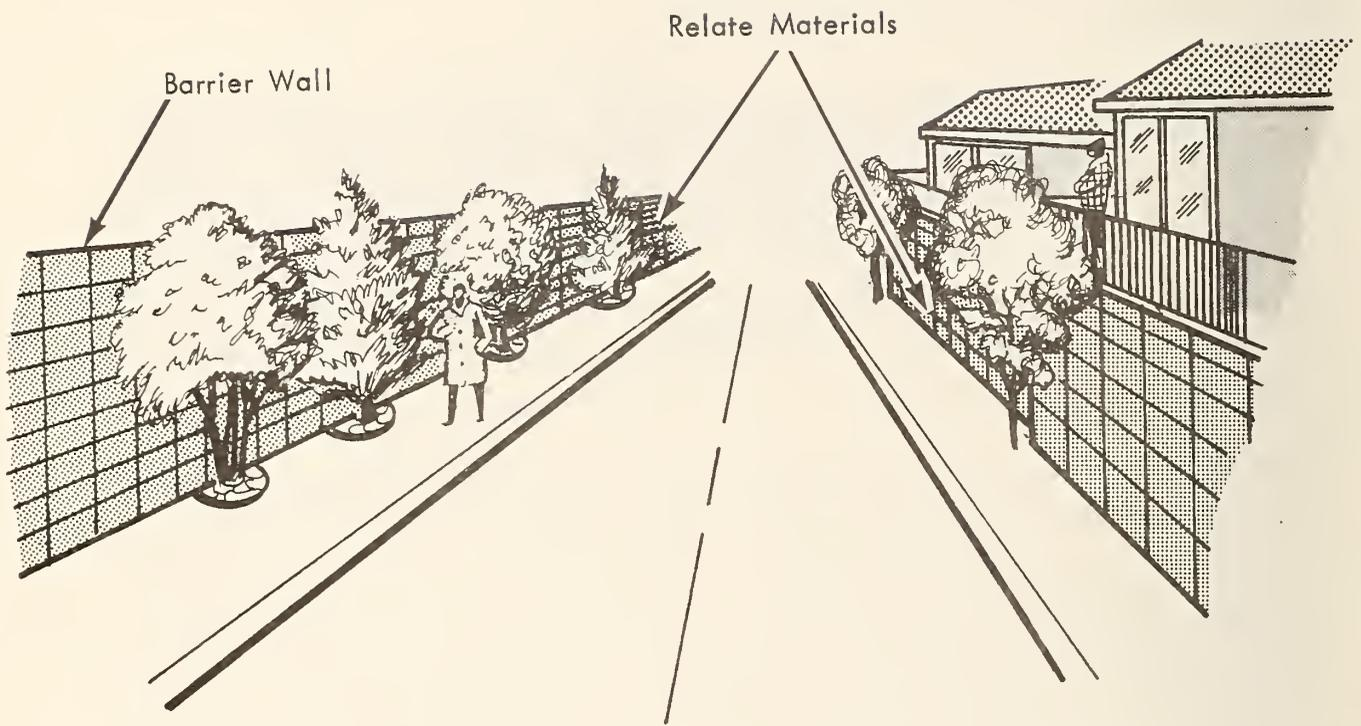
FIGURE 3-17. RELATING BARRIER DESIGN TO ARCHITECTURAL ELEMENTS IN THE COMMUNITY
