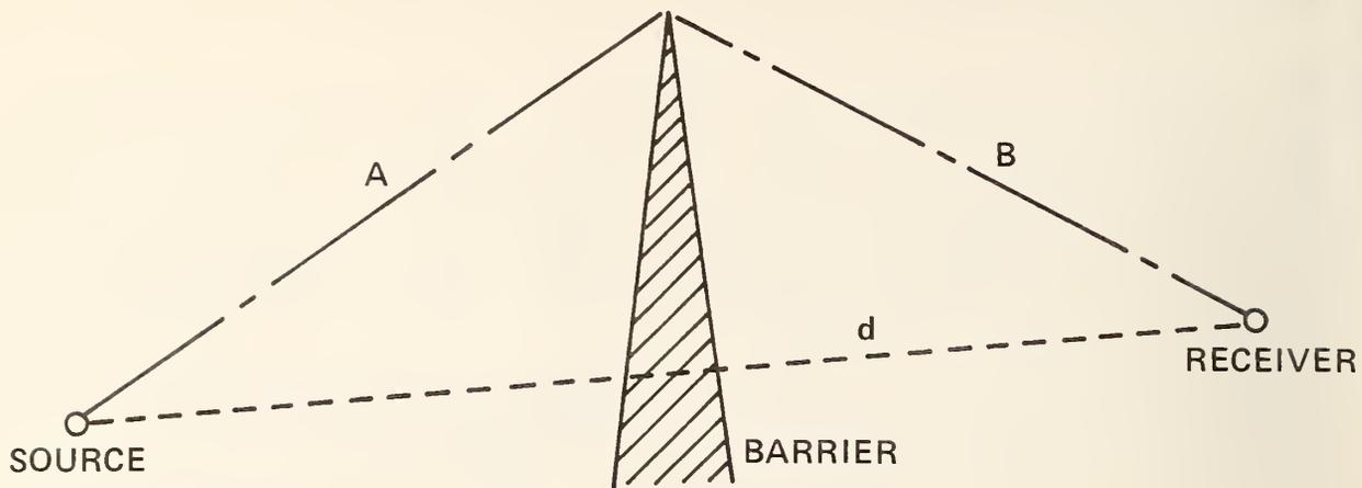
FIGURE 2-3 ILLUSTRATION OF PATH LENGTH DIFFERENCE.
