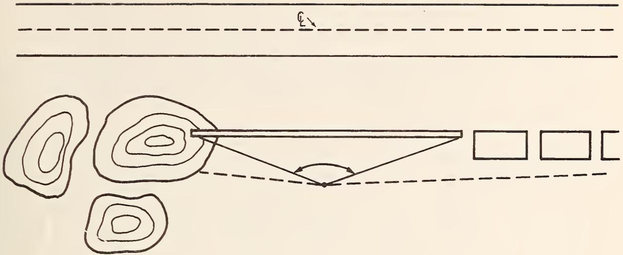
FIGURE 3-6 Use of Local Features to Achieve an "Infinite" Barrier.
