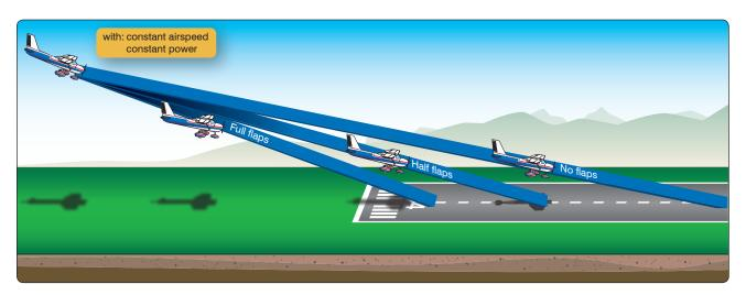
**Figure 8-3.** *Effect of flaps on the landing point.*
