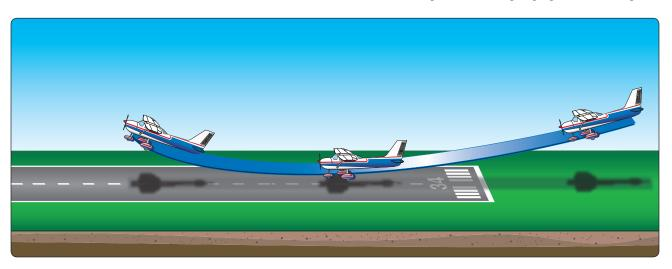
Figure 8-35. Ballooning during roundout.
