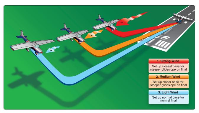
Figure 8-25. Plan the base leg for wind conditions.
