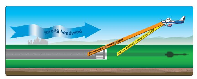
Figure 8-2. Effect of headwind on final approach.
