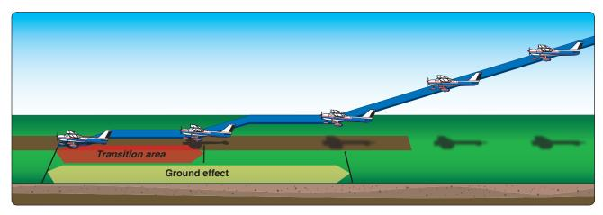
Figure 8-24. Soft/rough field approach and landing.
