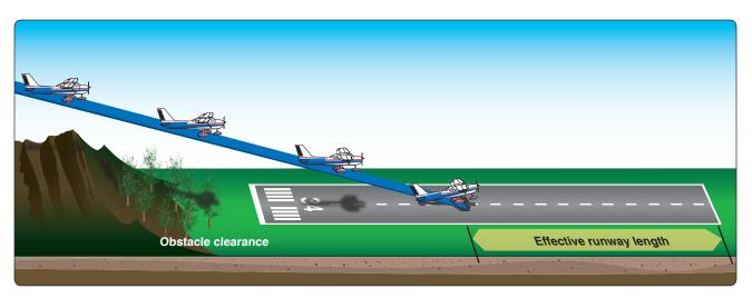
Figure 8-20. Landing over an obstacle.
