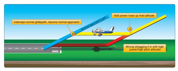
**Figure 8-31.** *Right and wrong methods of correction for low final approach.*
