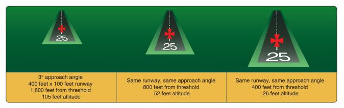
Figure 8-10. Runway shape during stabilized approach.
