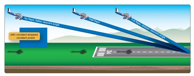
**Figure 8-4.** *Effect of flaps on the approach angle.*
