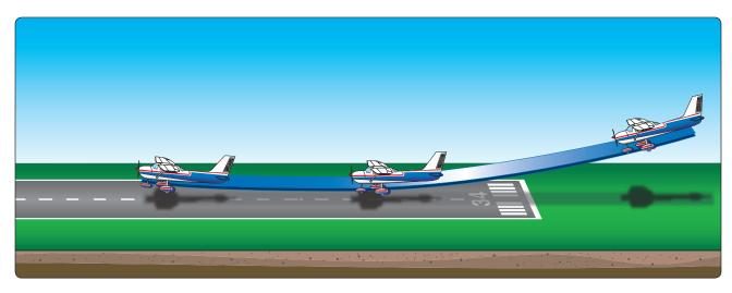
Figure 8-34. Floating during roundout.
