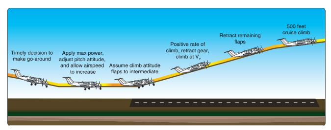
Figure 8-14. Go-around procedure.
