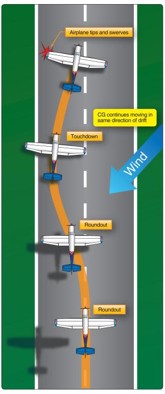
Figure 8-39. Start of a ground loop.
