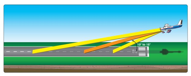
**Figure 8-7.** To obtain necessary visual cues, the pilot should look toward the runway at a shallow angle.
