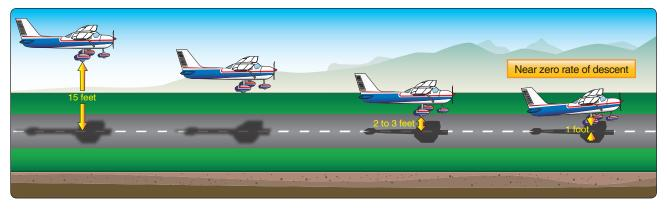
**Figure 8-8.** A well-executed roundout results in attaining the proper landing attitude.
