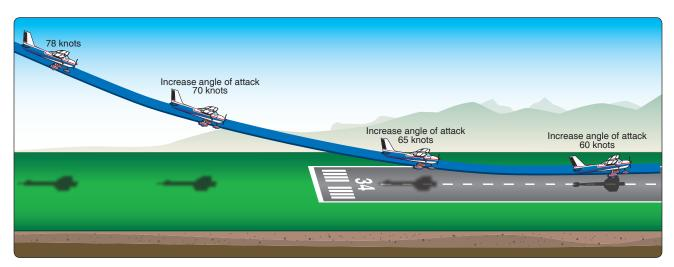
Figure 8-6. Changing angle of attack during roundout.
