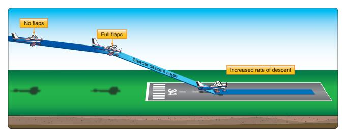
Figure 8-32. Change in glidepath and increase in descent rate for high final approach.
