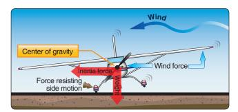
Figure 8-38. Drifting during touchdown.
