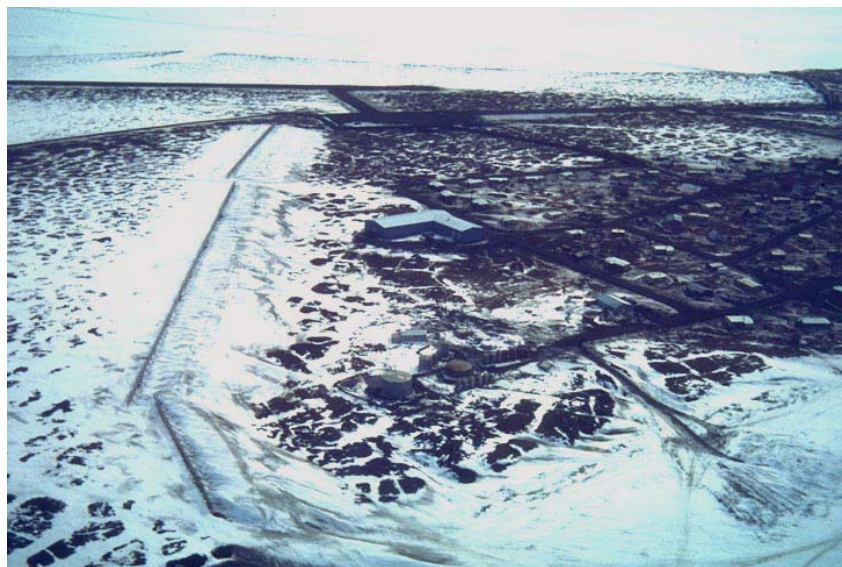
Figure 2.17. Conditions at Wainwright on Alaska's North Slope before (above) and after (right) a 4.6-m (15-ft) snow fence was built in 1982 (upper photo by Robert L. Jairell, U.S. Forest Service Research; photo right by Dr. Carl S. Benson, Geophysical Institute, University of Alaska -- Fairbanks). (From Tabler 1994).
