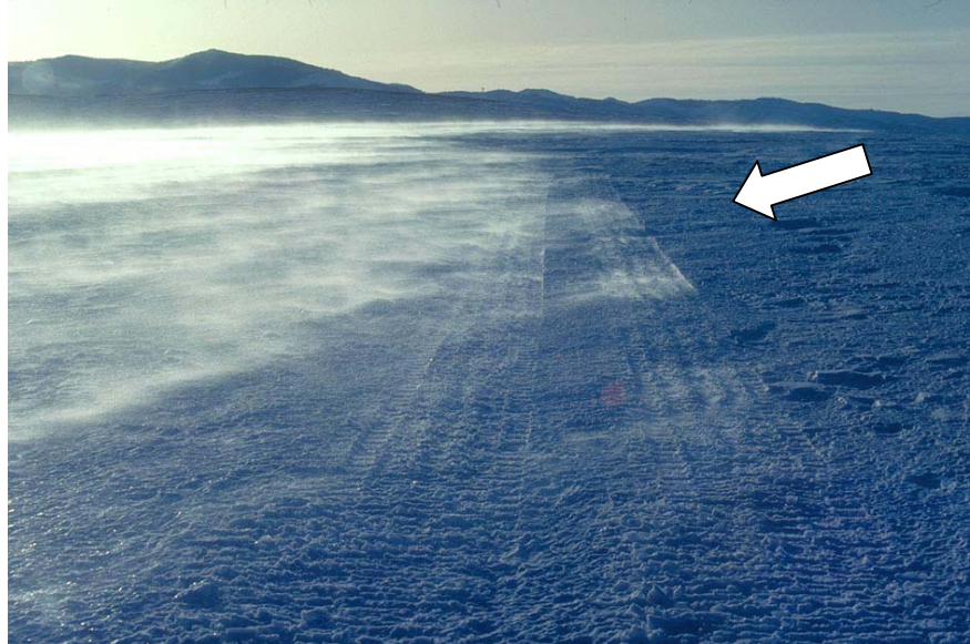
Figure 3.4. Chain reaction of saltating snow particles downwind from where tractor treads broke the snow crust (arrow indicates wind direction). Such disturbances act as sources of blowing snow that can persist over long distances downwind (Tabler 1986).
