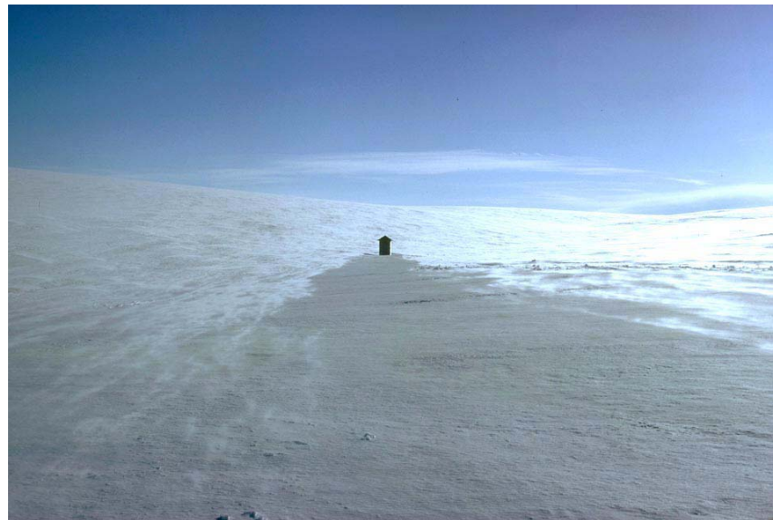
Figure 3.7. Snow shadow formed by a cylindrical shelter 1.2 m (4 ft) in diameter and 2.1 m (7 ft) tall (Tabler 1986). This view is from a point 150 m (500 ft) directly downwind. U. S. Forest Service photo by Robert L. Jairell.
