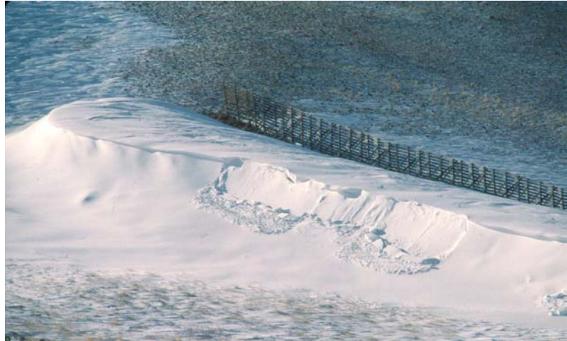
Figure 3.32. Slip face and cornice behind a 3.8-m (12.4-ft) snow fence (Tabler 1994). Drift is approximately 3.7 m deep at the cornice.
