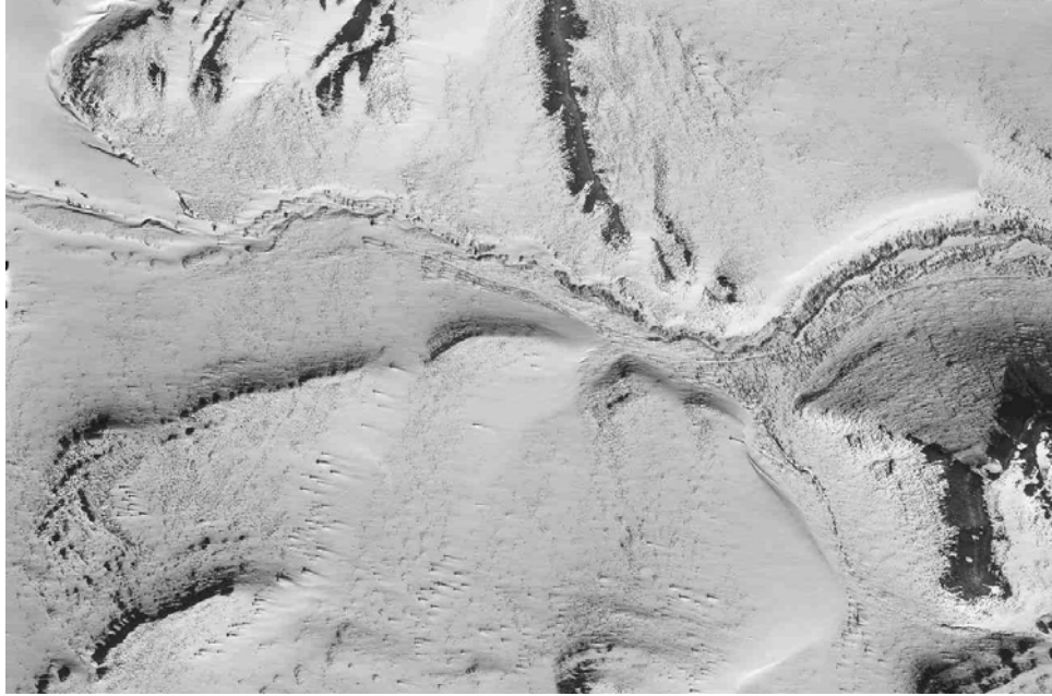
Figure 4.8. An aerial photo at a scale of 1:12000 shows alignment of drifts behind large shrubs and terrain features (Tabler 1986).
