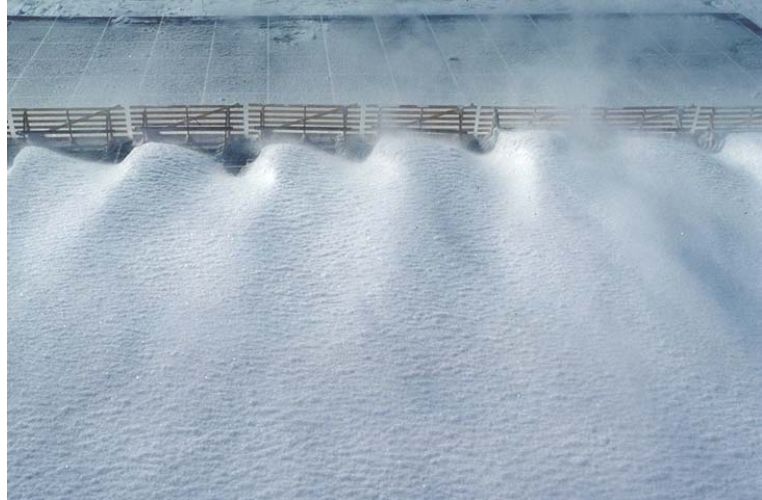
Figure 6.82. Model of a 1.8-m-tall (6-ft) Wyoming fence with 15-cm-wide (6 in.) boards on 30-cm (12 in.) centers (facing wind). Note how leaving 15-cm (6-in.) gaps between panels reduces fence effectiveness.
