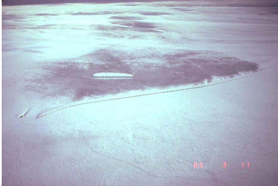
Figure 2.18. This aerial view downwind shows that the effect of a snow fence can extend for great distances downwind (Tabler 1994). A 3.8-m (12-ft-tall) fence in the foreground is trapping most of the incoming snow. The increased eroding capability of the wind has scoured out snow for nearly a kilometer downwind. The shorter fence in the snow-free area was used to measure the snow trapping efficiency of the main fence. U.S. Forest Service Photo by A. Loren Ward.
