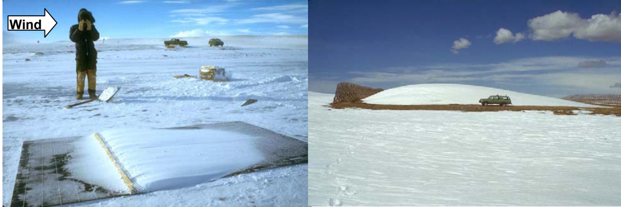
Figure 3.40. Equilibrium drift formed by a 6-cm (2.4-in.) reduced-scale model of a 1.8-m (6-ft) fence (left) is proportional to that formed by a 3.8-m (12.4 ft) fence (Tabler 1986).
