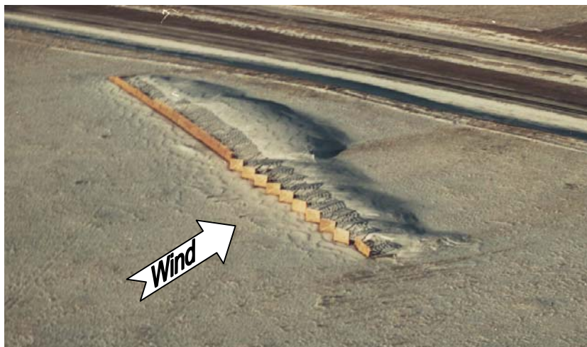
Figure 6.22. Aerial view shows zigzag design catches less snow than the standard Wyoming fence with which it was paired for comparison (Tabler 1986b). Fence height is 3.8 m (12.5 ft). Photo by Robert L. Jairell. From Tabler (1994).
