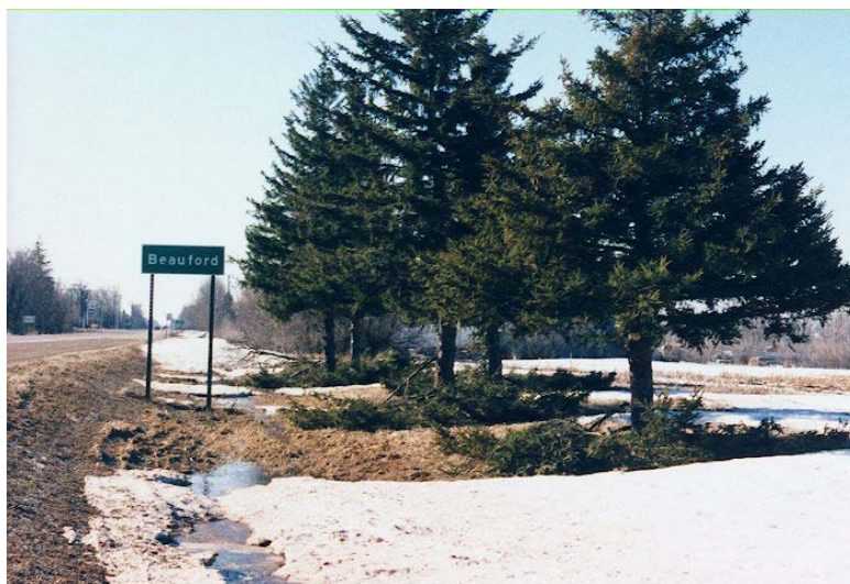
Figure 5.35. Pruning lower branches of roadside trees can mitigate snow drifting problems.
