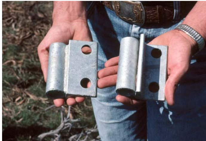
Figure 6.17. Anchor attachment for permafrost soils allows fence to move vertically in response to thawing and freezing of active layer. Dimensions are in millimeters.
