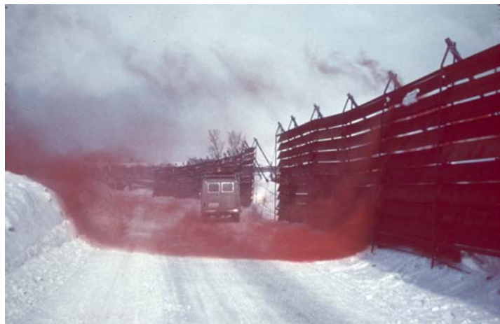
Figure 6.65. Smoke was used to show the airflow behind typical blower fence used in Japan to reduce snow blowing off roadside snow banks at windshield level, with wind from right (Tabler 1986b). Photograph courtesy Tetsuya Uchiya, Hokkaido Development Bureau.
