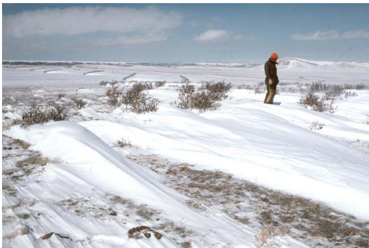
Figure 4.6. The orientation of streamlined drifts formed by bushes and trees can be used to determine the prevailing direction of the snow transport (Tabler 1994).
