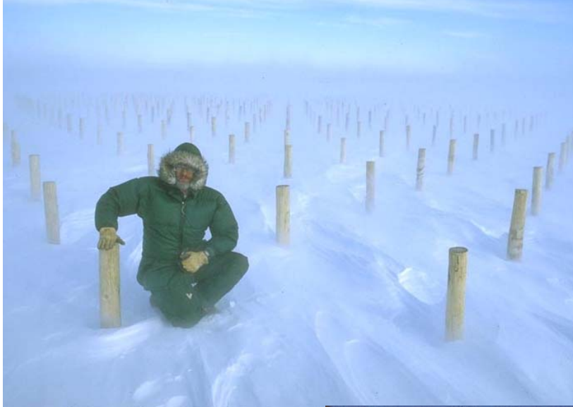
Figure 3.23. Snow retained in a field of posts 130 mm (5 in.) in diameter, 1.2 m (4 ft) tall at different spacings illustrates how the geometry of surface roughness controls snow deposition (Tabler 1994).
