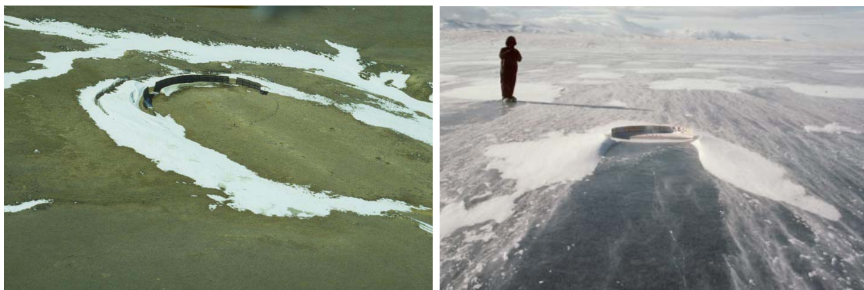
Figure 6.67. Aerial view of drift pattern around livestock shelter (left, photo by R. L. Jairell). A 1:30 scale model of this shelter (right) illustrates the effectiveness of lateral deflectors in preventing snow deposition on the downwind side, and the wing-shaped drifts that form along the side of the wake (Tabler 1986b).
