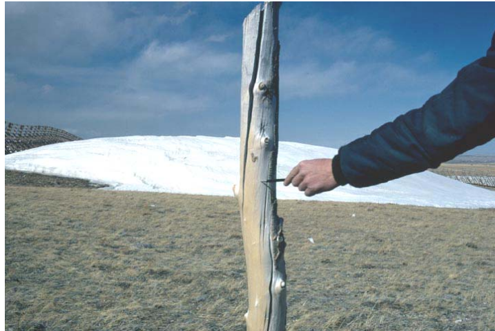
Figure 4.7. Abrasion pattern on posts indicates prevailing direction of snow transport (Tabler 1986).
