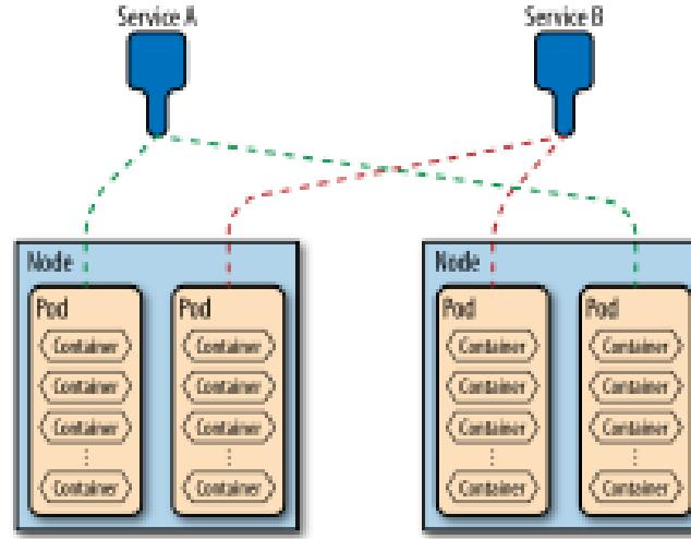
An endpoint that provides load balancing across a replicated group of pods
