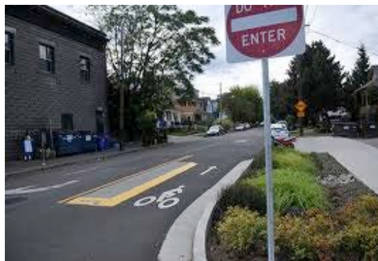
Bicycle-friendly streets should incorporate curb extensions, green infrastructure, and other traffic calming features to create a comfortable walking/bicycling environment.
