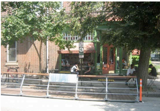
Railings, curbs, or bollards should be used to protect flexible parking lane uses from errant vehicles.
