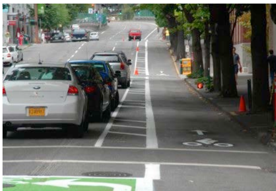
Cycle tracks may be separated from adjacent travel lanes using parking lanes, raised pavement, planters, or other treatments.
