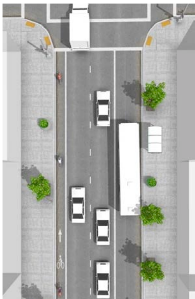
Typical left-side bike lane design (NACTO)
