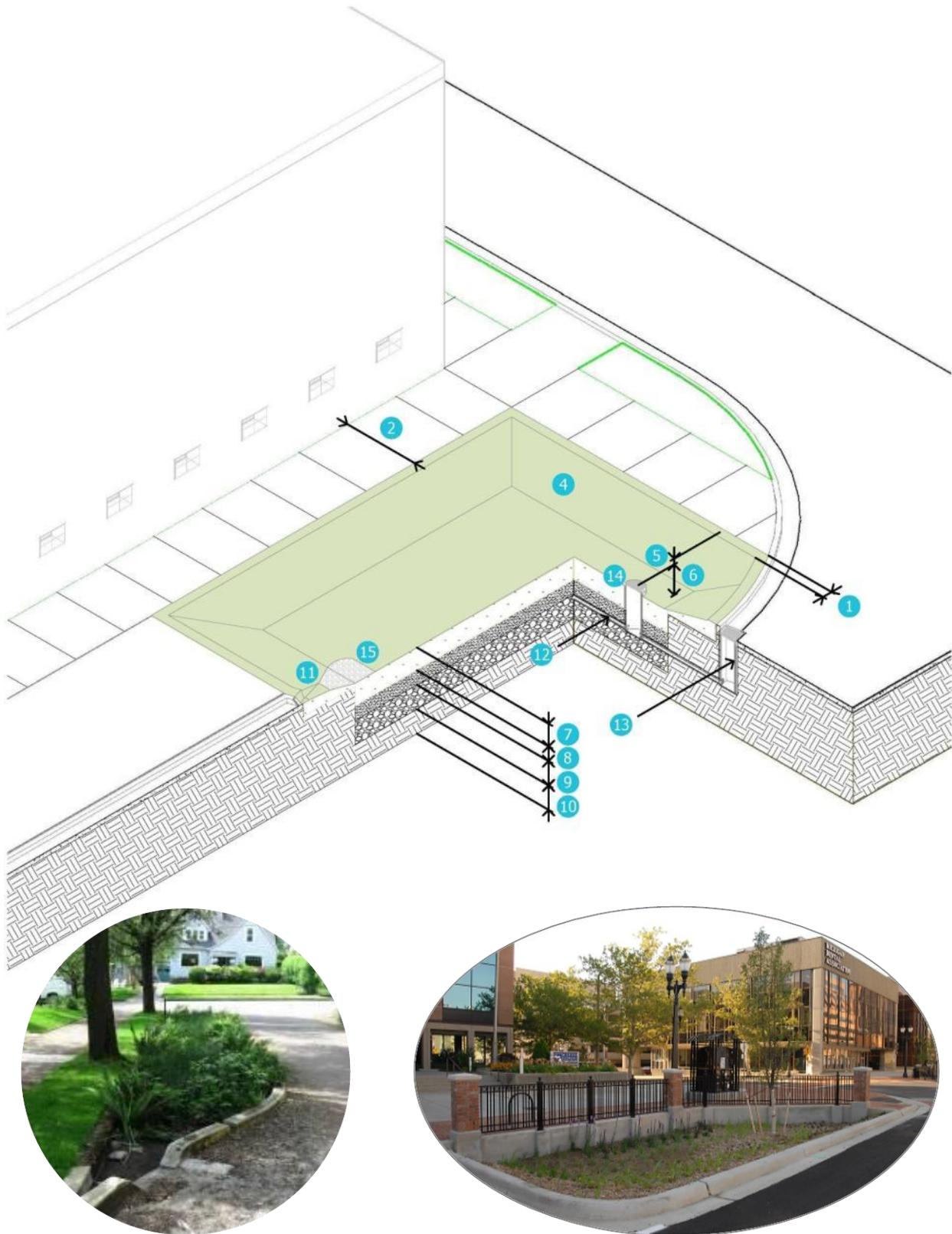
**FIGURE 5-9 BIORETENTION CURB EXTENSION DIAGRAM**
