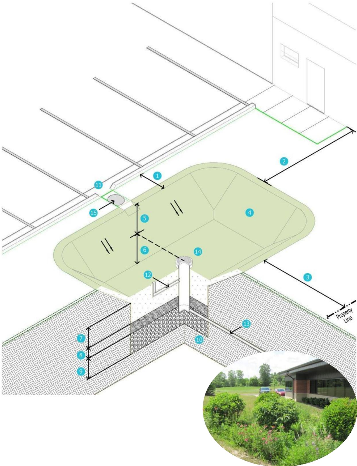
**FIGURE 5-5 TRADITIONAL BIORETENTION DIAGRAM**
