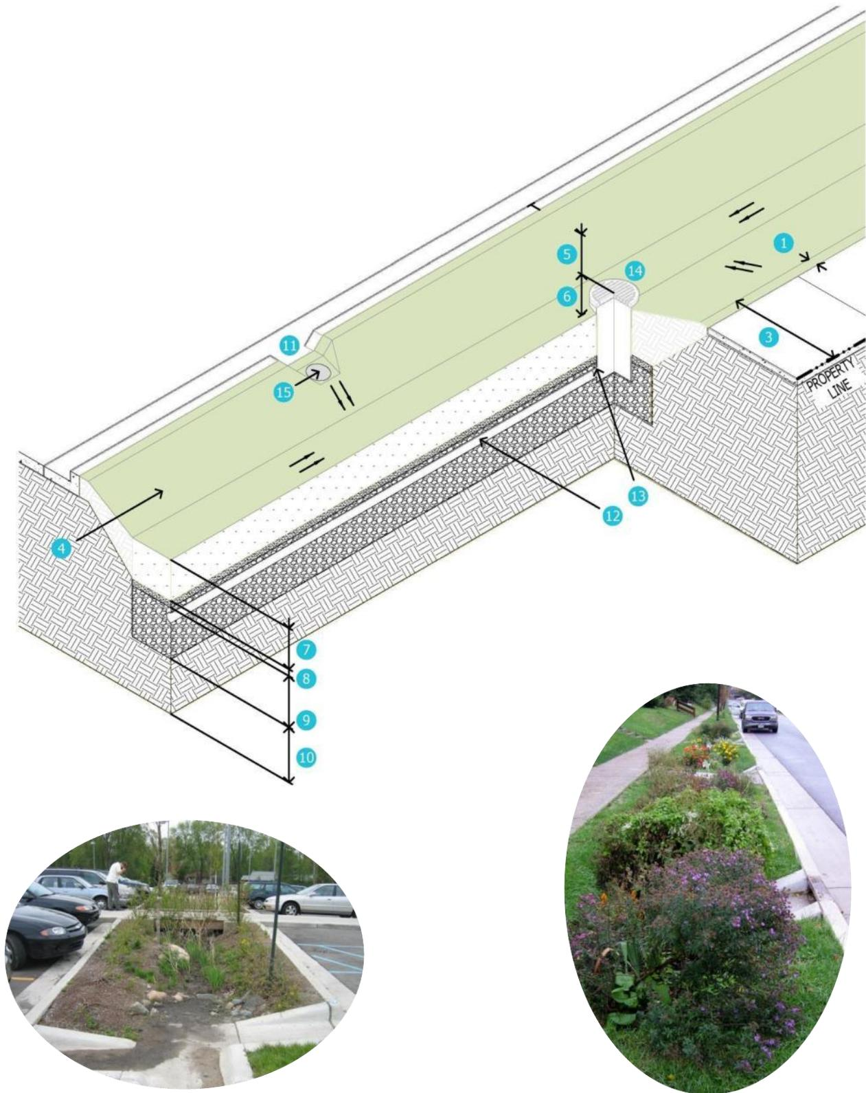
**FIGURE 5-6 BIORETENTION SWALE DIAGRAM**
