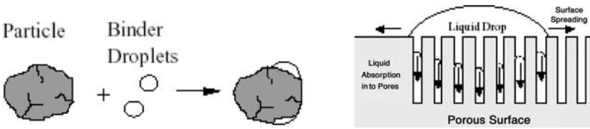
Figure 13 Stages of wetting for coarse powder compared to drop size. (From Ref. 5.)
