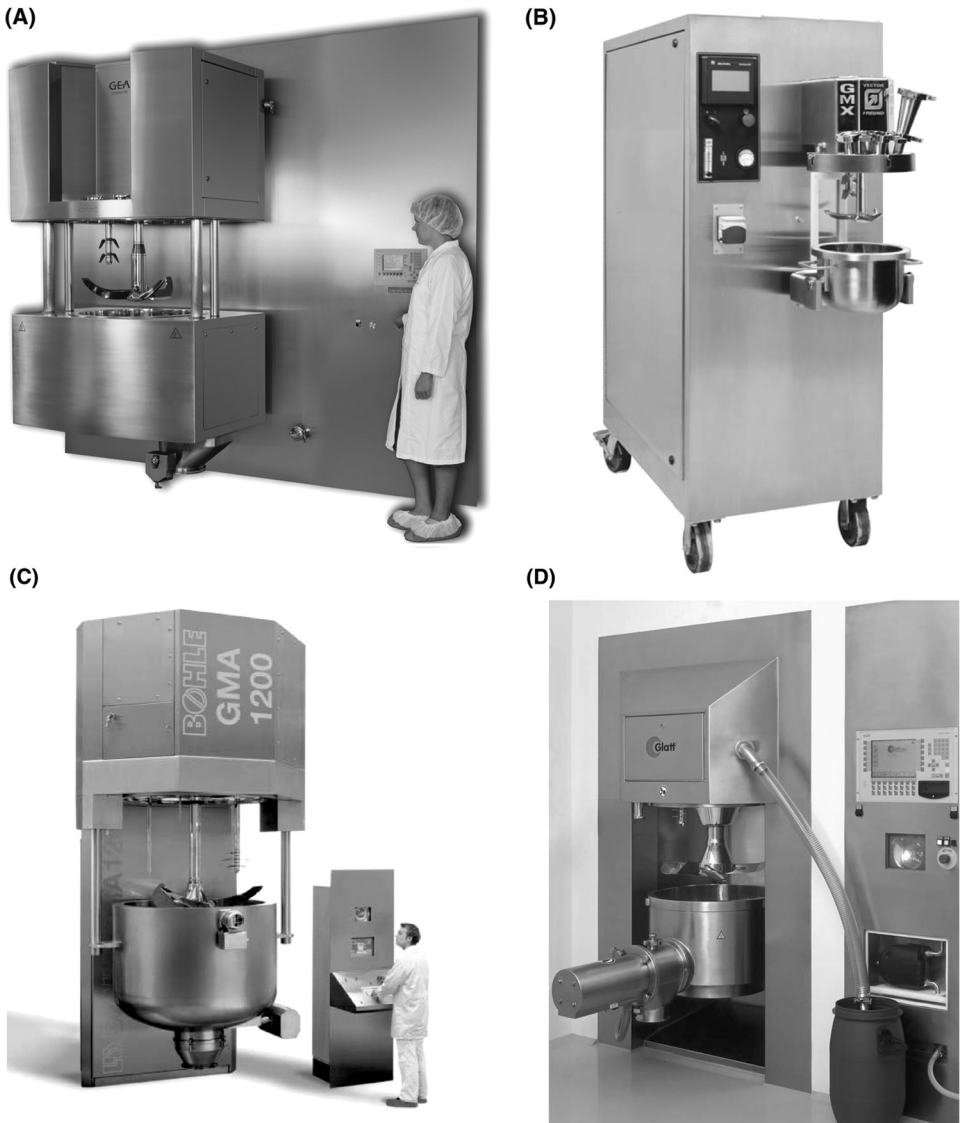
Figure 3 (A) Photograph of a top-driven vertical high shear granulator (UltimaGral 150). (Courtesy of Niro Pharma Systems.) (B) Photograph of a top-driven vertical high shear granulator. (GMX 10 courtesy of Vector Corporation.) (C) Photograph of a top-driven vertical high shear granulator. (GMA 1200 courtesy of L. B. Bohle.) (D) Photograph of a top-driven vertical high shear granulator. (Courtesy of Glatt Air Techniques.)
