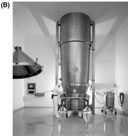
Figure 26 (A) PLC based system. (Courtesy of Niro Pharma Systems.) (B) Production unit with a PLC control panel. (Courtesy of the L.B. Bohle Group.)
