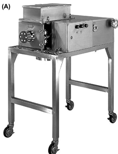
Figure 1 Oscillating granulator: (A) Frewitt MF line and (B) rotor, screen, and tensioning spindles.
