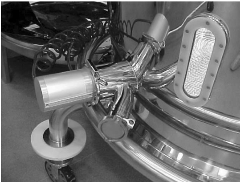
Figure 39 (A) Side discharge. (Courtesy of the Glatt Group.) (B) Side discharge. (Courtesy of Niro Pharma Systems.)
