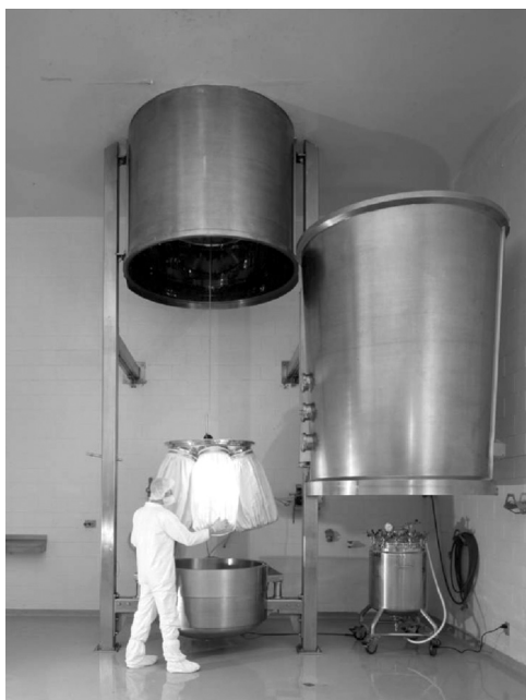
Figure 13 Production size unit with filter bags. (Courtesy of the L.B. Bohle Group.)
