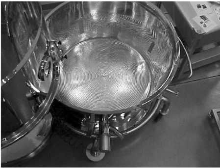
Figure 6 (A) Schematic of the overlap gill plate—gill arrangements. (B) Container with the overlap gill distributor. (Courtesy of Niro Pharma Systems.)
