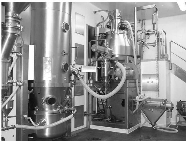
Figure 35 Loading of fluid bed from high-shear mixer. (Courtesy of the Glatt Group.)
