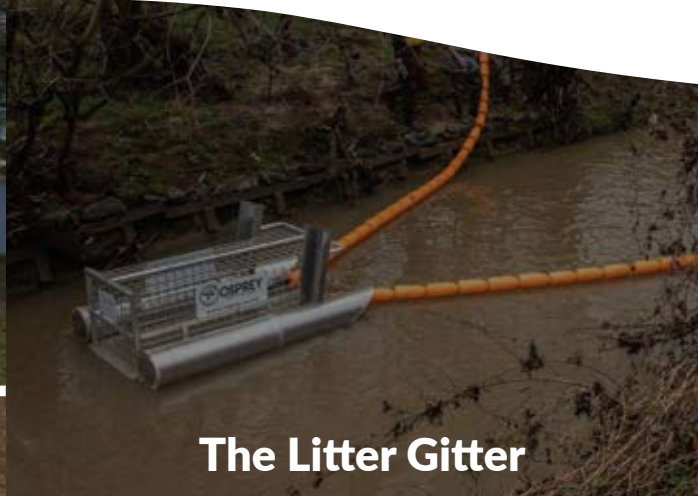
This patented technology prevents the downstream flow of floating litter. Initial tests indicate an 80+% success rate.
