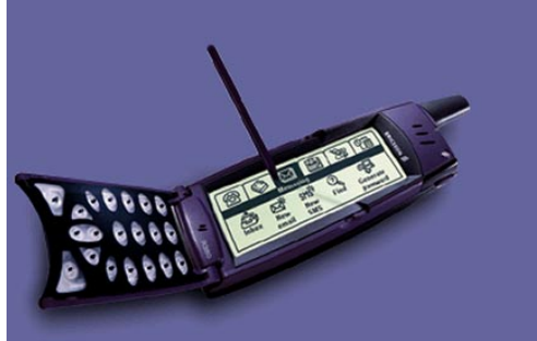
Fig. 10.7 Ericsson R380 phone, which uses the EPOC operating system. (Courtesy of Ericsson.)
