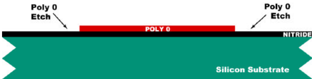
Figure 1.4. Reactive ion etching (RIE) is used to remove the unwanted polysilicon. After the etch, the photoresist is chemically stripped in a solvent bath. This method of patterning the wafers with photoresist, etching and stripping the remaining photoresist is used repeatedly in the MUMPs™ process.
