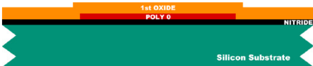
Figure 1.5. A 2.0 μm layer of PSG is deposited on the wafers by low pressure chemical vapor deposition (LPCVD). This is the first sacrificial layer.
