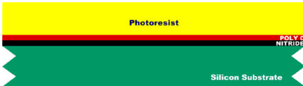
Figure 1.2. The surface of the starting n-type (100) wafers are heavily doped with phosphorus in a standard diffusion furnace using POCI 3 as the dopant source. A 600 nm blanket layer of low stress silicon nitride (Nitride) is deposited followed by a blanket layer of 500 nm polysilicon (Poly 0). The wafers are then coated with UV-sensitive photoresist.
