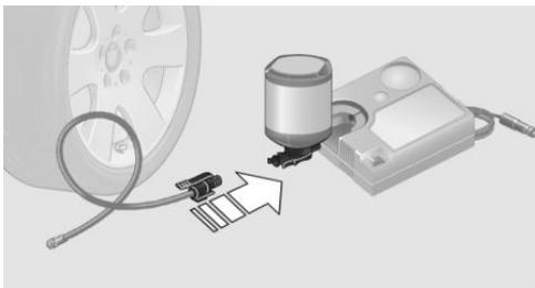
4. Slide the sealing container upright into the holder on the compressor housing, ensuring that it engages audibly.
