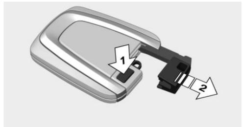
Press button, arrow 1, and remove the key, arrow 2.
