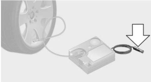
5. Correct the tire inflation pressure to 2.5 bar.
