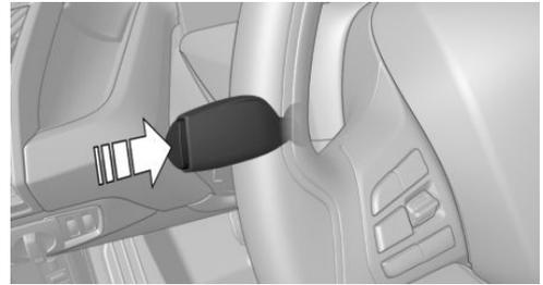
Press the onboard computer button on the turn signal lever.
