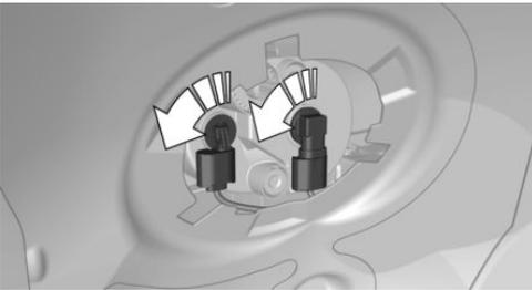
2. Press the bulb gently into the socket, turn counterclockwise and remove.
