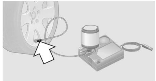
6. With the compressor switched off, insert the plug into a power socket inside the vehicle.
