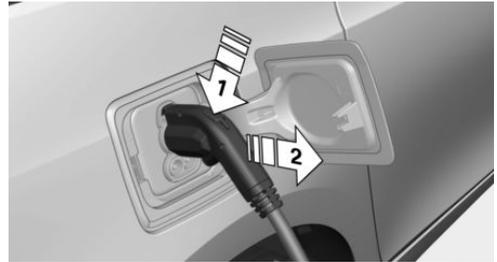
3. Remove the charging cable from the charging port, arrow 2.
