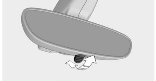
To reduce the blinding effect of the interior rear view mirror, flip the lever forward.
