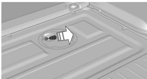
6. Carefully insert the dipstick up to the stop in the measuring tube, and pull it back out. The engine oil level must be between the two marks of the dipstick.
