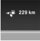
The total range considers the capacity of the fuel tank as well as the electric energy in the high-voltage battery.
