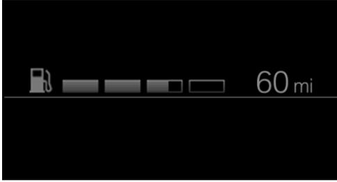
The fill level bars indicate the available fuel supply of the Range Extender when operating readiness and drive readiness are switched on.
