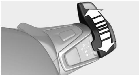
Turn the selector lever in the desired direction. The engaged selector lever position is displayed on the selector lever.
