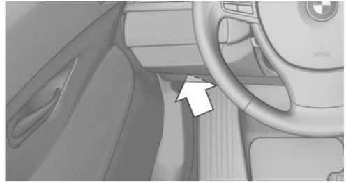
Located on the driver's side is an OBD socket for reading the vehicle data. On vehicles with Range Extender, additional components are checked that are critical for its emissions mix.
