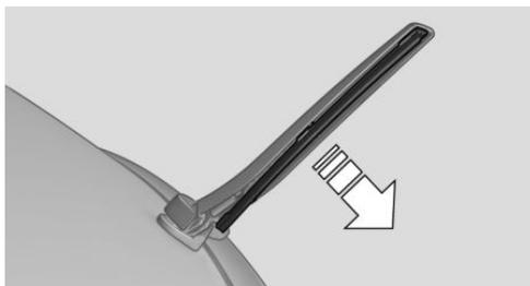
2. Attach a new wiper blade. It must engage audibly.
