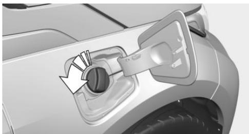
5. Fuel the vehicle as usual. This may be difficult due to the residue pressure in the tank, caused by frequent stopping of the fuel pump nozzle, e.g.
