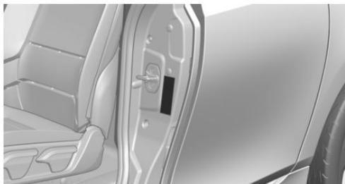
These pressure values can also be found on the tire inflation pressure label on the driver's side on the rear door.
