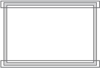
Use two insertion profiles running parallel to the long side frame.
