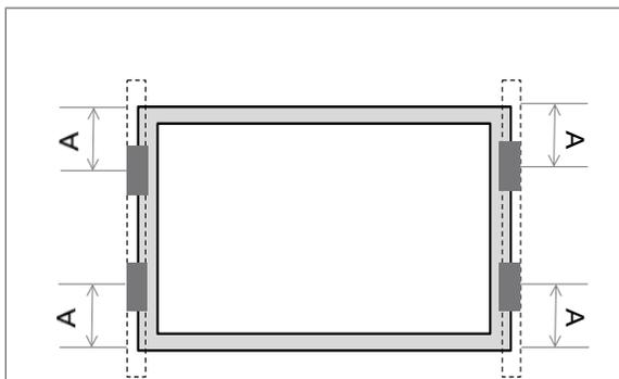
Use four clamps on the short side. Mounting rails run perpendicular to the long side frame.
