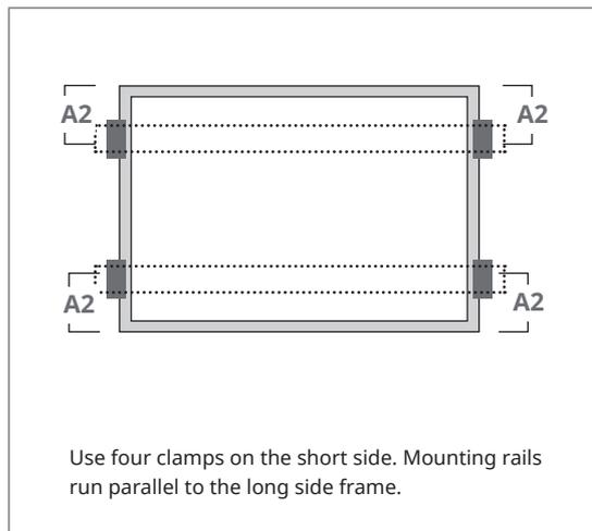
Use four clamps on the short side. Mounting rails run parallel to the long side frame.
