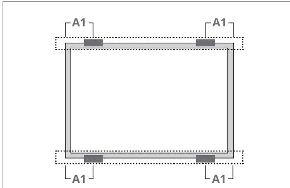
Use four clamps on the long side. Mounting rails run parallel to the long side frame.
