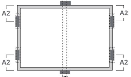
Use four clamps on the short side and two clamps on the long side. An additional support bar should be placed below the center of the module.
