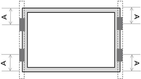
Use four clamps on the short side. Mounting rails run perpendicular to the long side frame.
