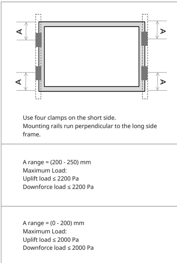
**Rail-less clamping for CS3K-P, CS3K-MS, CS6K-P,
