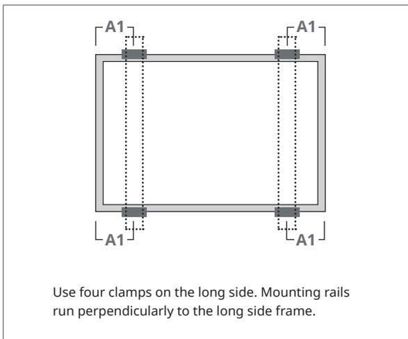
Use four clamps on the long side. Mounting rails run perpendicular to the long side frame.
