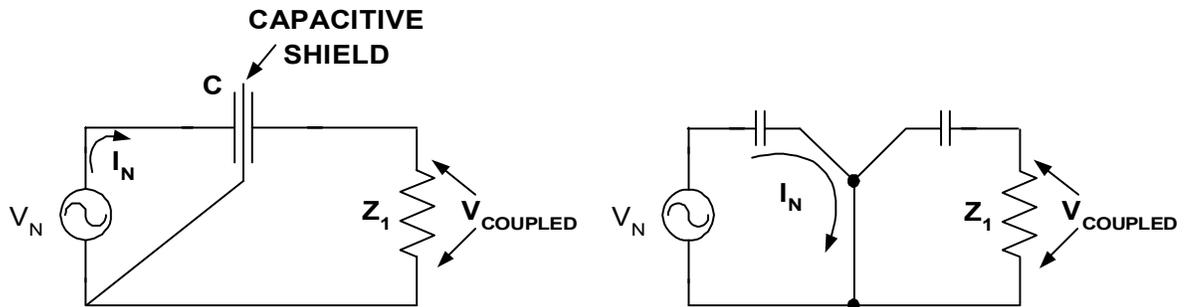
**Figure 12.26:** An Operational Model of a Faraday Shield
