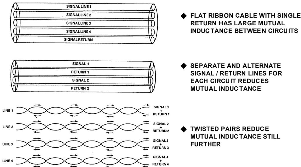
**Figure 12.22:** Mutual Inductance and Coupling Within Signal Cabling
