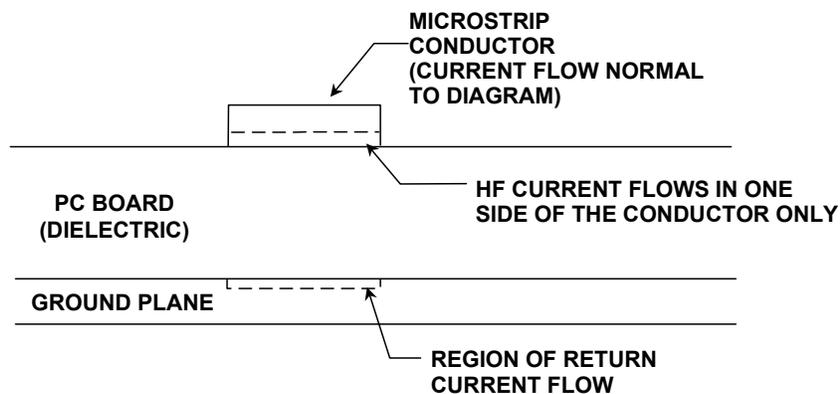
**Figure 12.32:** Skin Depth in a PCB Conductor
