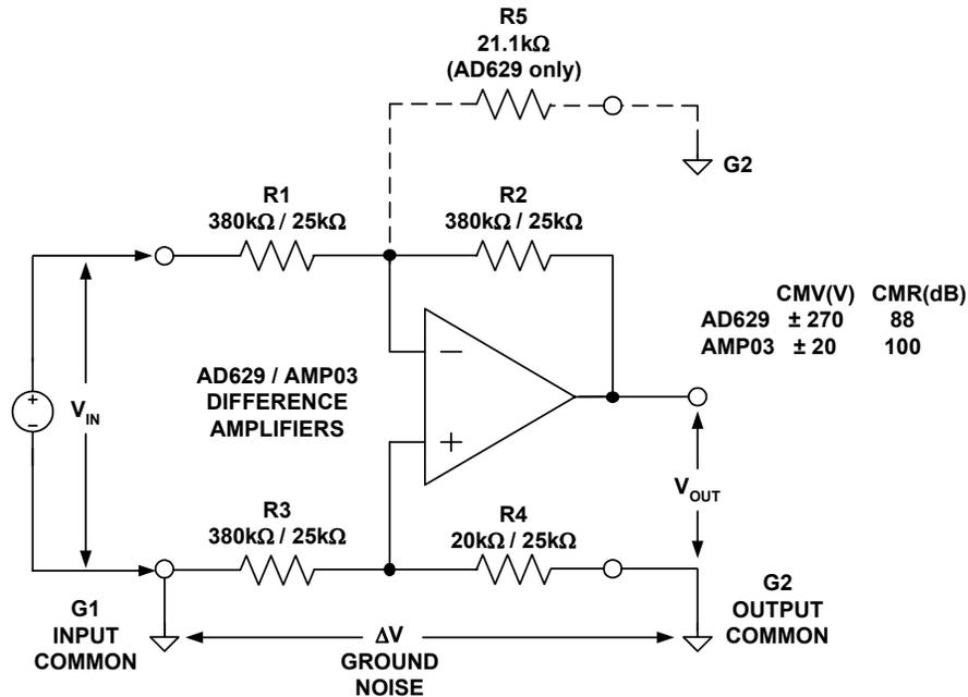
**Figure 12.11:** A Differential Input Ground Isolating Amplifier Allows High Transmission Accuracy by Rejecting Ground Noise Voltage Between Source (G1) and Measurement (G2) Grounds
