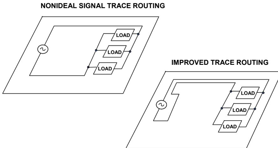
**Figure 12.19:** *Nonideal and Improved Signal Trace Routing*
