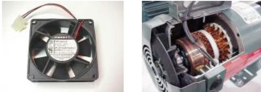
Two examples of DC motors – the picture on the right is cut open to show the windings. You can find more information on motors at http://my.execpc.com/~rhadley/magmotor.htm
