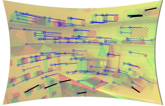
Figure 6: Example on real images. Matches selected as inliers for  $F$  (Left) and  $F \& \lambda$  (Right, distortion corrected via the calculated  $\lambda$ ).  $F$  gives 130 matches plus 4 outliers, while the new model gives 140 matches, 1 outlier, and places the new matches (thicker tracks on the right) towards the periphery of the image.
