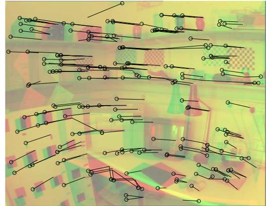
Figure 7: Using a artificially high threshold (4 pixels), the traditional fix for  $F$  estimation with distortion. More inliers are obtained but at the expense of including false matches.
