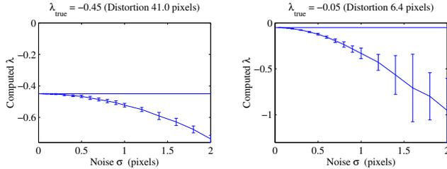
Figure 4: Tests on synthetic data. Synthetic image size is  $640 \times 480$ , and plausible 3D data are obtained by using stereo reconstruction from a real scene. The graphs show the computed distortion coefficient  $\lambda$  as a function of noise level on the 2D points. The horizontal line is the nominal value. A systematic bias to high corrections is evident, and is more pronounced on images with less distortion. Compare this to linear ellipse fitting.
