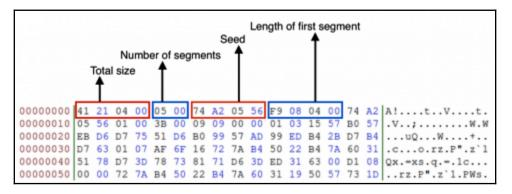
Figure 35: The structure used for decryption in the Vawtrak malware
