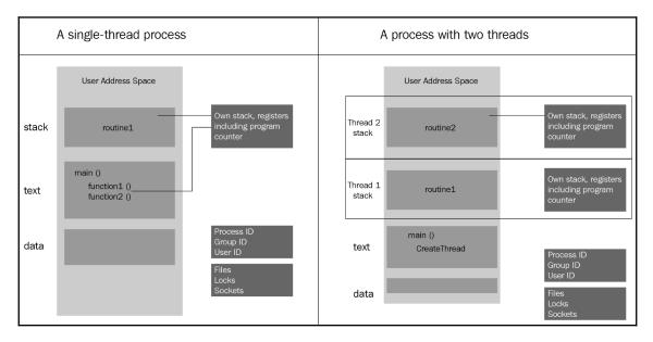
Figure 12: Example processes with one and multiple threads
