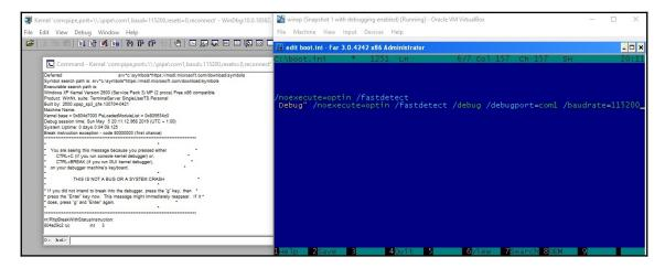
Figure 21: Kernel-mode debugging with VirtualBox and WinDbg over port COM
