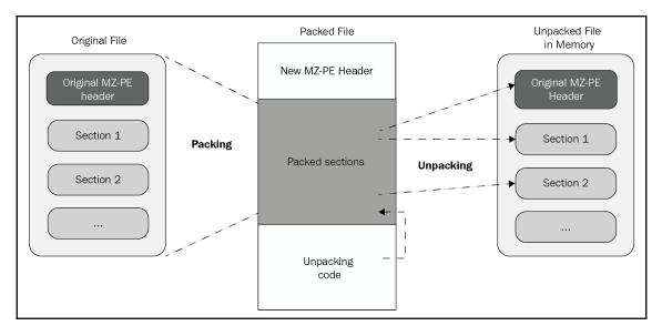
Figure 1: The process of unpacking a sample
