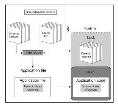
Figure 8: Dynamic linking from compilation to loading
