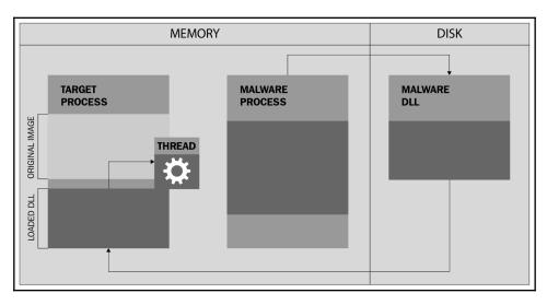
Figure 3. Simple DLL injection mechanism
