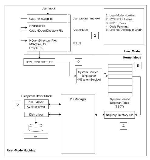
Figure 6: The hooking mechanisms of rootkits
