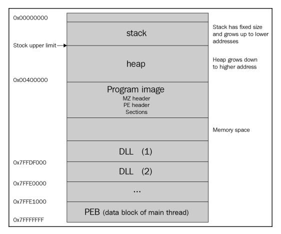
Figure 10: Example of a 32-bit process memory layout
