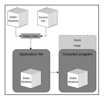
Figure 7: Static linking from compilation to loading
