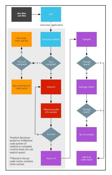
Figure 5: The process of compiling and executing files in ART
