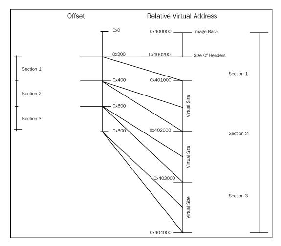
Figure 13: Mapping sections from disk to memory
