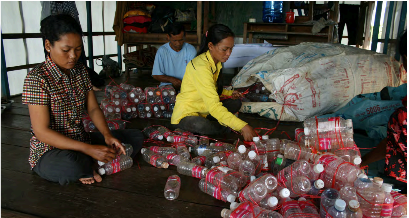
In prototype 1, small water bottles are tied into groups of four, before packing the into rice sacks.
