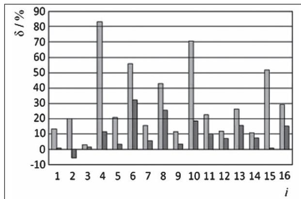
**Figure 14** Maximal and minimal errors for component weights  $i$  during automatic dosing
