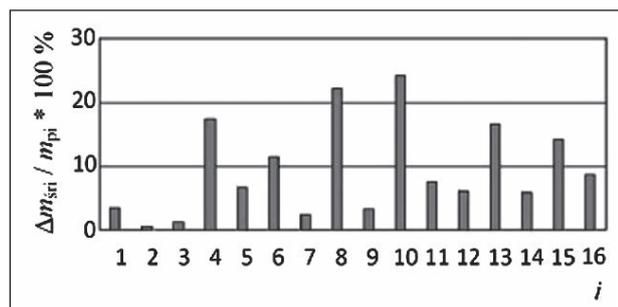
**Figure 13** Errors for component weights  $i$  during automatic dosing
