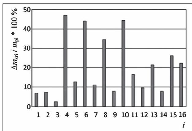
**Figure 12** Errors for component weights  $i$  during semi-automatic dosing
