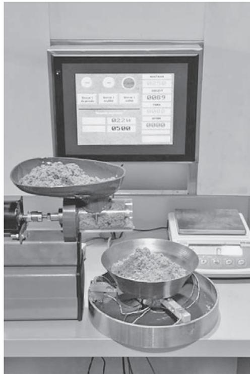
Figure 8 The dispensing model system stand
