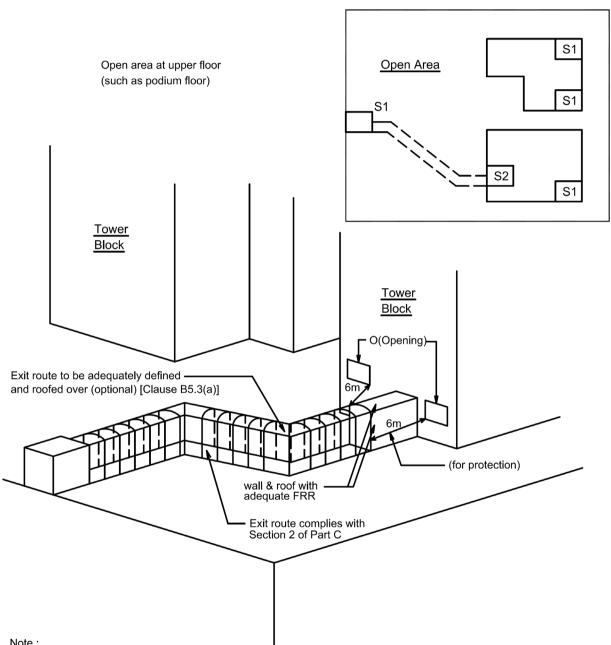
The exit route across the open area should be designed and constructed as if it is part of the protected exit.
