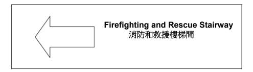
The height of the words and characters on the notice should be not less than 20mm. Such notice should be either illuminated by two separate systems of electric light or a type of safety sign which is self-energized in respect of luminosity and which requires no external source of power.
