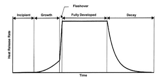
Diagram G2: Typical Phases of a Fire Curve
