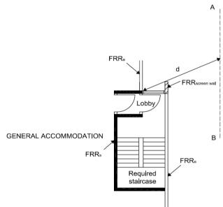
FRRe: FRR of the external wall FRRs: FRR of the required staircase
