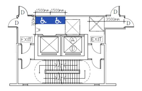
Lobby to fireman's lift of minimum dimensions of 1.5m to be used as wheelchair manoeuvring space
