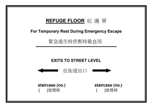
(c) Sufficient directional signs in the following form should be displayed at appropriate positions at the refuge floor at a height of 1500mm above the floor level, to indicate the direction of travel in order to enter the respective required staircase;
