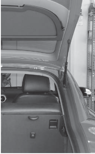
(a) A roof strut that holds open a car hatch.
