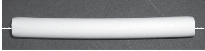
(a) Chalk before applied torque exceeds critical value.
