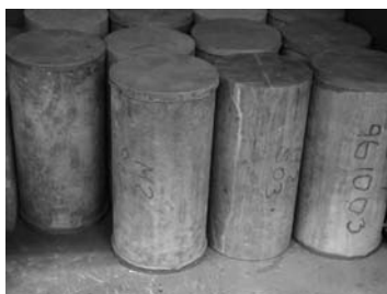
Fig. 2.8 Test specimen for testing the compressive properties of concrete; they are 6 by 12 inches.
