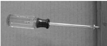
Fig. 7.2 Both the screwdriver shaft and the screw are loaded in torsion when driving the screw into the wood member.
