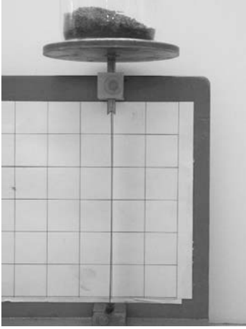
Fig. 12.14 Pin-pin beam subject to a load below the buckling load.
