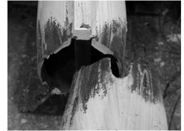
Fig. 2.25 A steel pipe that has been pulled in tension beyond its ultimate stress point.
