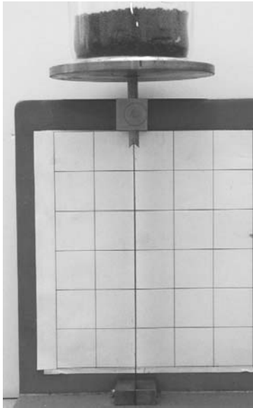
Fig. 12.1 Pin-clamped beam subject to a load below the buckling load.
