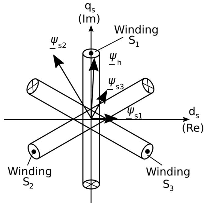
**Figure 82: Flux linkage of a three-phase system (5)**
