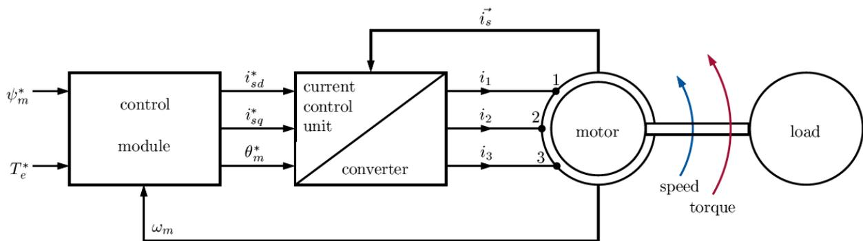
**Figure 92: Field-oriented control drive structure (7)**
