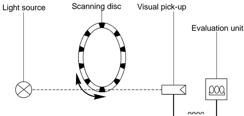
**Figure 84: Optical incremental position encoder (5)**
