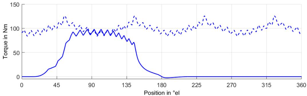
**Figure 58: Torque production of a four phase SRM (5)**
