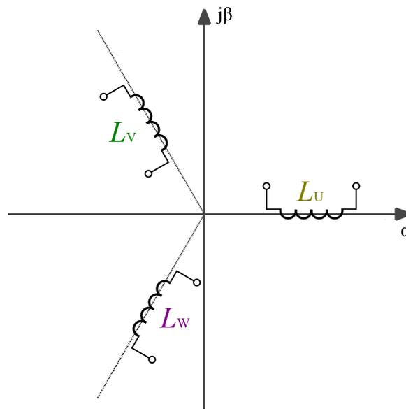
**Figure 90: Arrangement of the  $\alpha\beta$ -coordinate system (48)**
