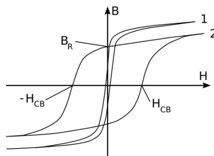
**Figure 97: B(H)-characteristic of magnetic materials (5) (55)**
