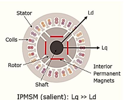
**Figure 20: Cross section of a salient externally excited synchronous machine [left], non-salient surface mounted permanent synchronous machine (PMSM/SMPMSM) [center] and a salient interior permanent magnet machine (IPMSM) [right]**
