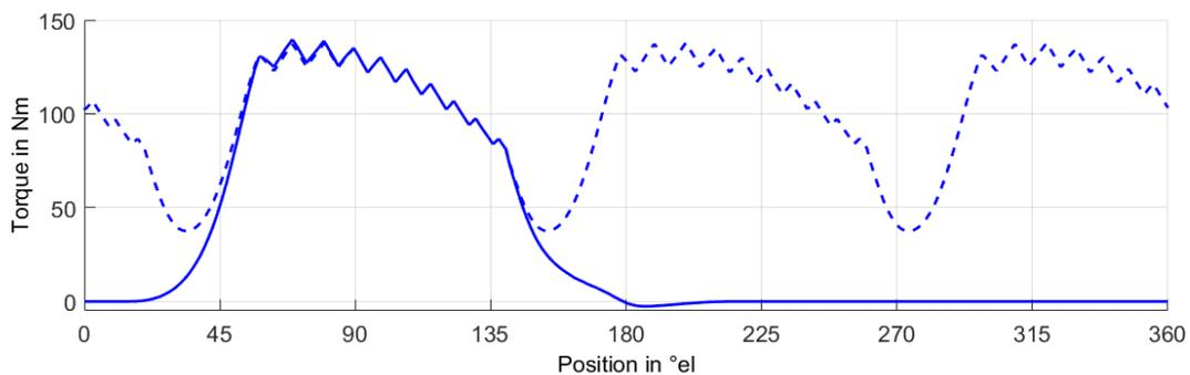
**Figure 57: Torque production of a three-phase SRM (5)**
