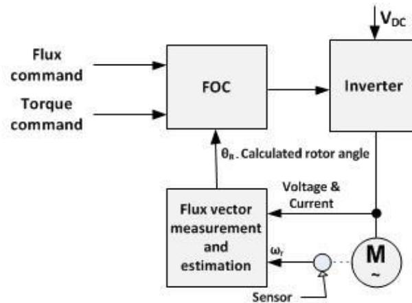
**Figure 94: Block diagram of direct field-oriented control (DFOC) (50)**
