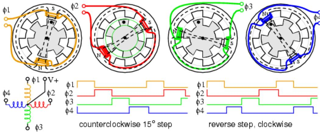
**Figure 62: Stepping sequence for variable reluctance stepper (31)**
