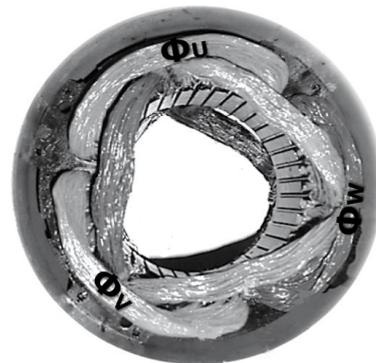
**Figure 2: Distributed winding inside stator**
