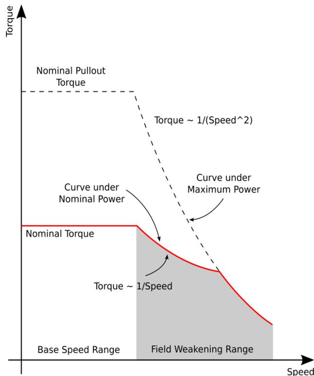
**Figure 13: Operating range of the induction motor (5)**
