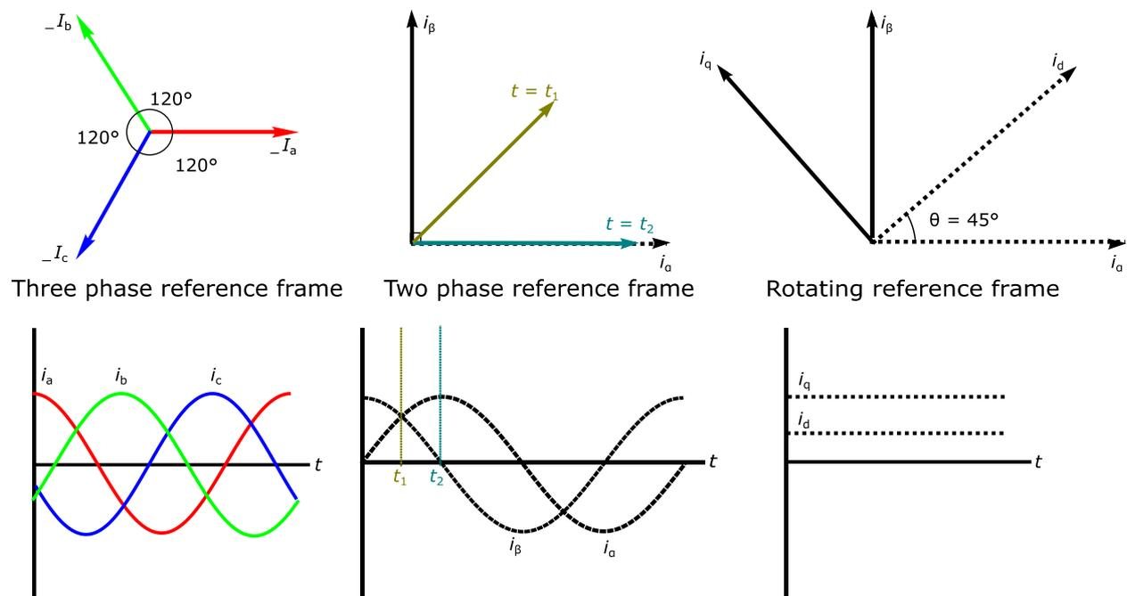
**Figure 91: Transformations of a three-phase system (5)**
