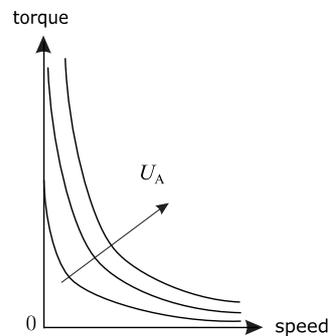
**Figure 35: Torque-speed characteristic curve of the series wound machine (5)**
