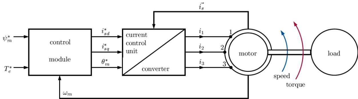
**Figure 92: Field-oriented control drive structure (7)**
