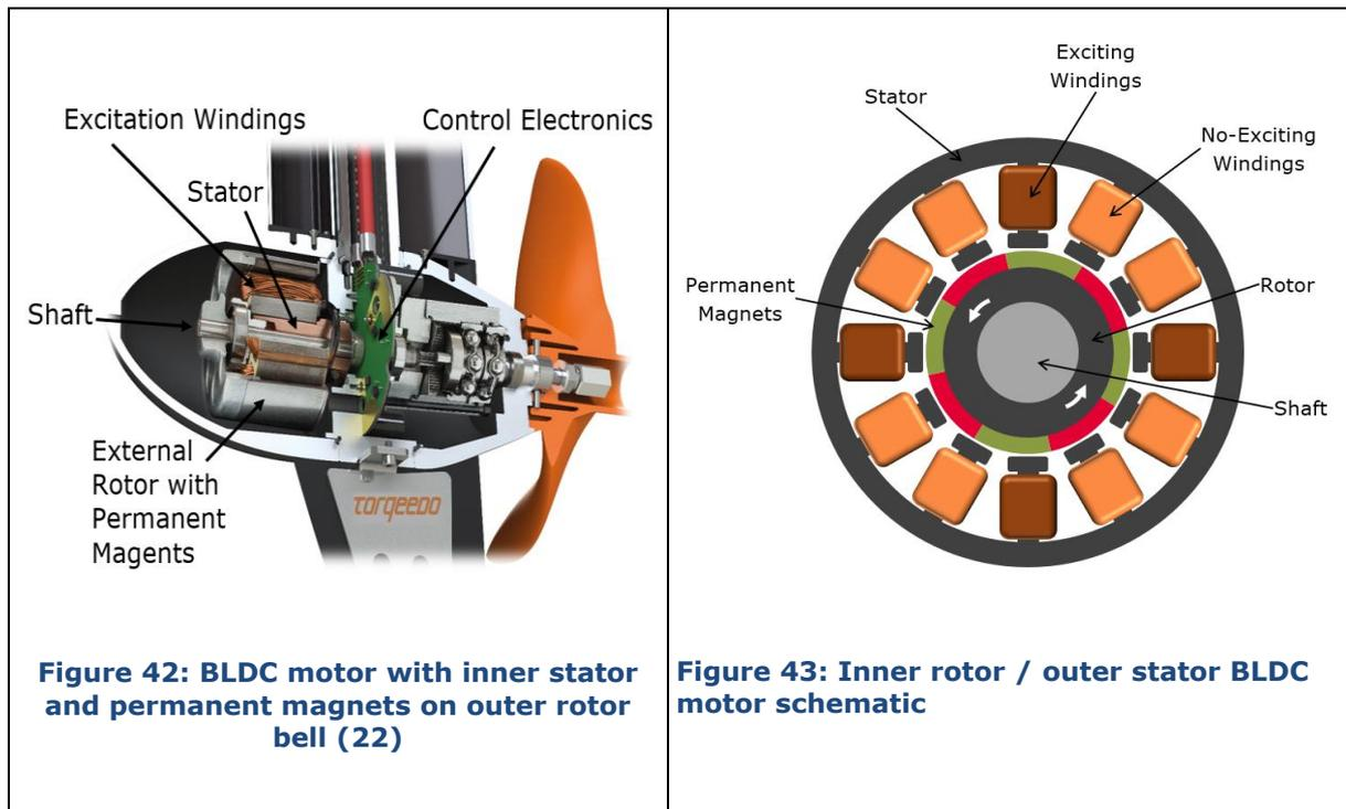
The essential difference to the conventional DC machine is that the commutation is performed electronically by a controller rather than mechanically by brushes. The windings are connected to a control circuit, which energizes the windings such that a rotating field is generated. The rotor magnet tries to align with the stator field providing torque and thus motion (23).
