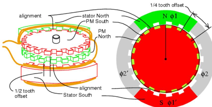
**Figure 70: Simplification of hybrid stepper motor (31)**
