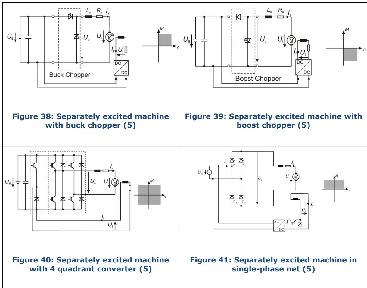
If a boost chopper is used, the DC machine can only be operated as a generator (
