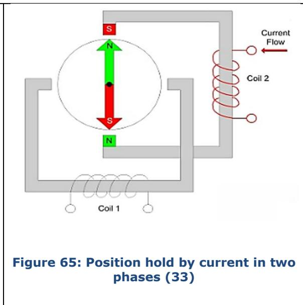
**Figure 65: Position hold by current in two phases (33)**
