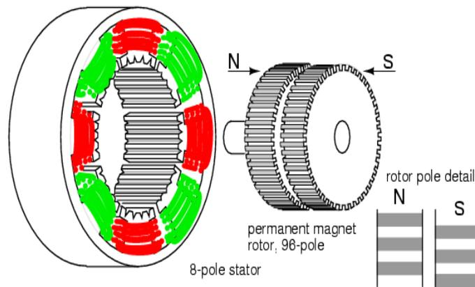
**Figure 69: Hybrid synchronous stepper motor (31)**
