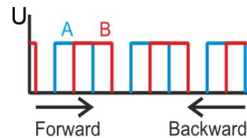
**Figure 86: Magnetic incremental position encoder (electrical pulses) (5)**
