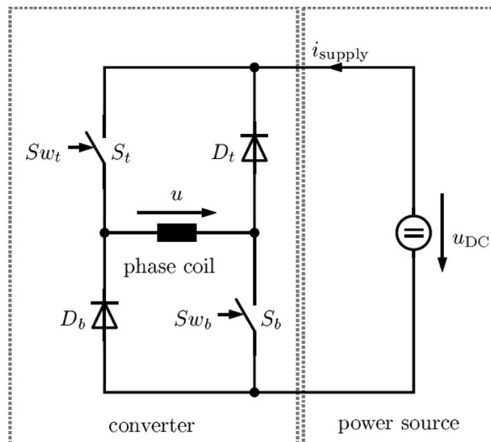
**Figure 50: SR drive with asymmetric half-bridge converter topology (7; 5)**
