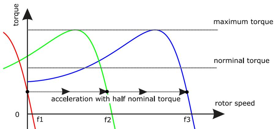
**Figure 11: Torque for V/f control (5)**
