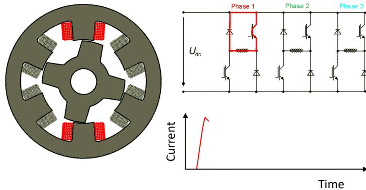
**Figure 52: Current flow of the free-wheeling state (5)**
