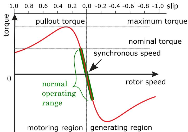
**Figure 6: Torque-vs.-speed diagram of the IM (5)**
