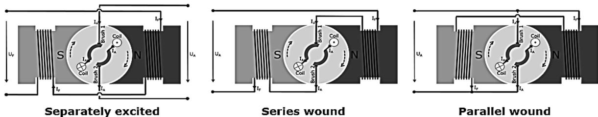
**Figure 31: Overview of the three different DC-motor types**
