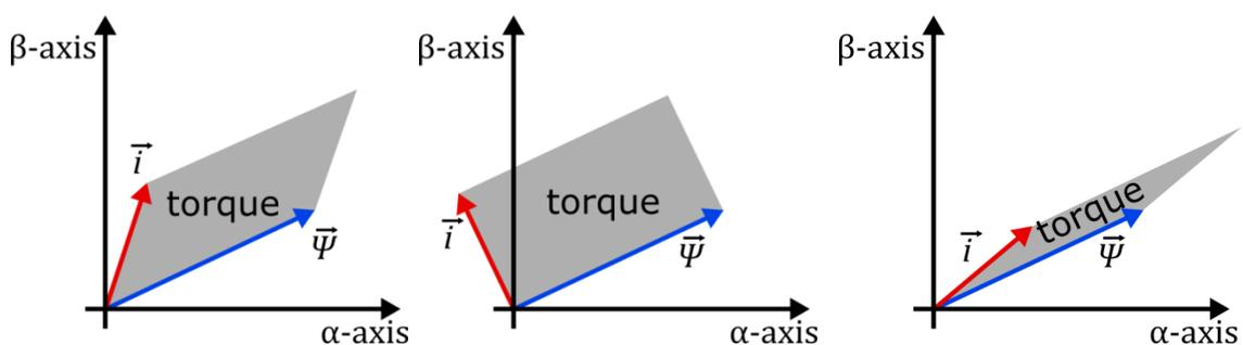
**Figure 79: Relationship between current / flux linkage space vectors and torque (5)**
