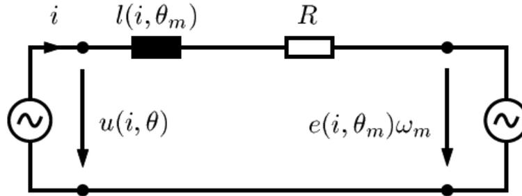
**Figure 49: Equivalent circuit of one phase of a switched reluctance machine (7)**
