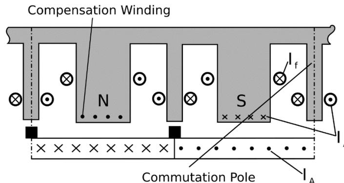
**Figure 30: Compensation windings and commutation pole of a separately excited DC machine (5)**
