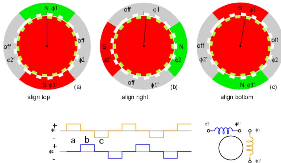
**Figure 71: Hybrid stepper motor rotation sequence (31)**
