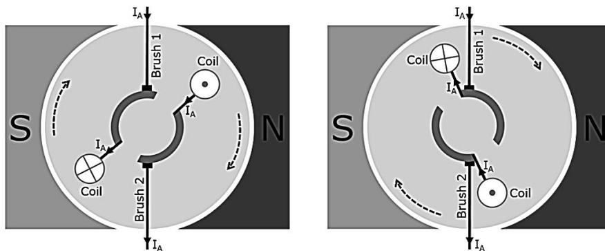
**Figure 28: Simplified cross section of a permanent magnet DC machine with two possible commutator positions, right after (left) and shortly before (right) next commutation**
