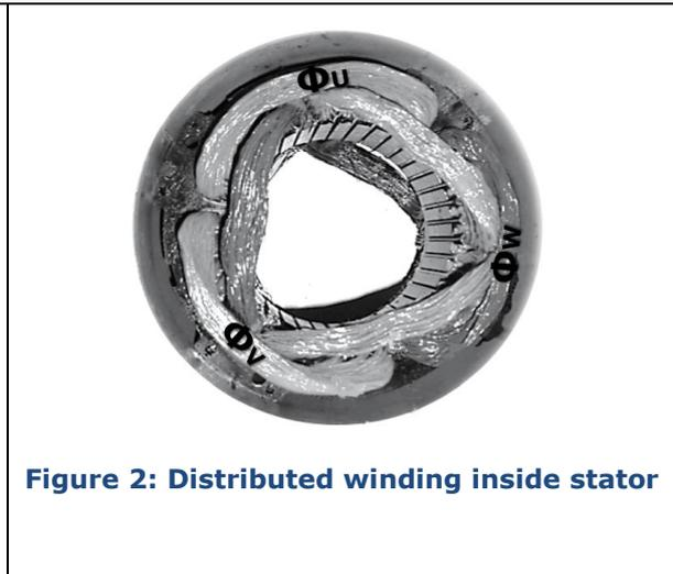
**Figure 2: Distributed winding inside stator**
