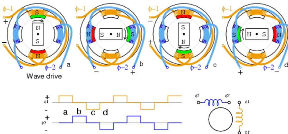
**Figure 66: Simplified permanent magnet stepper in wave drive (31)**
