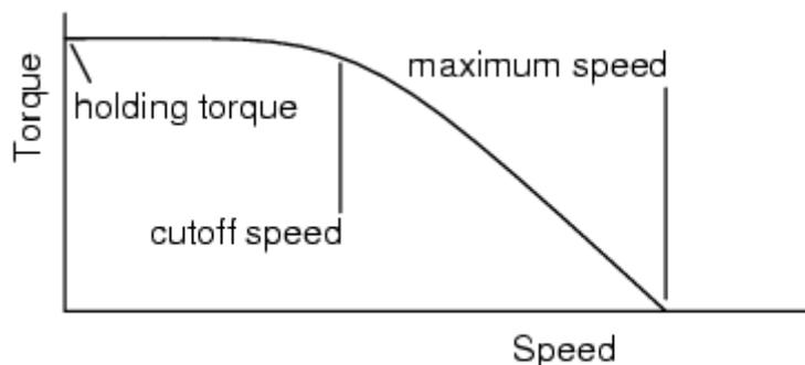
**Figure 74: Speed torque characteristics (31)**
