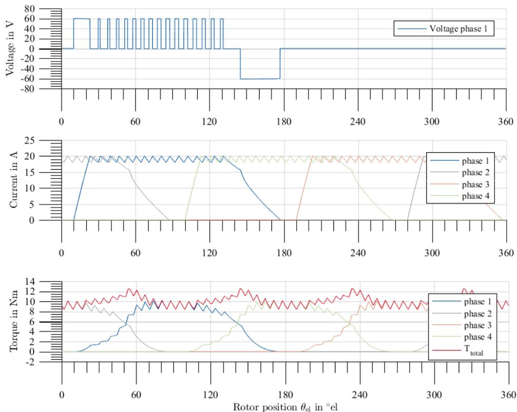
**Figure 55: Operating in low speed (7; 5)**
