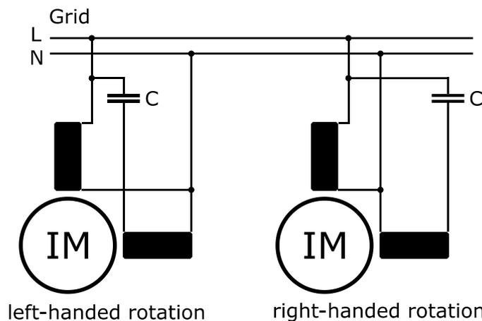
**Figure 18: One-phase induction motor as capacitor motor (5)**
