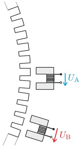
**Figure 85: Magnetic incremental position encoder (schematic) (5)**
