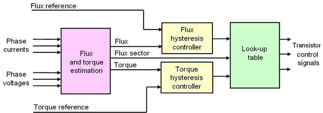
**Figure 95: Block diagram of direct torque control (DTC) (52)**
