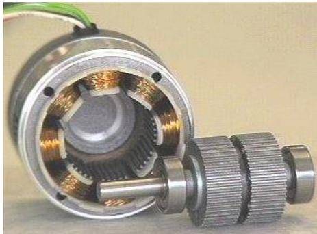
**Figure 59: Hybrid synchronous stepper motor (28)**
