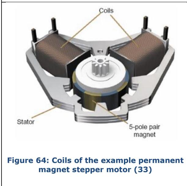
**Figure 64: Coils of the example permanent magnet stepper motor (33)**
