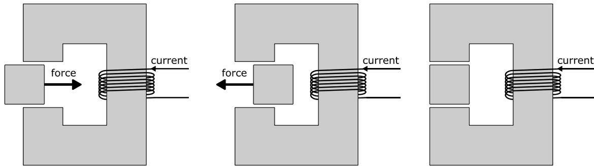
**Figure 80: Reluctance force in a magnetic circuit (5)**
