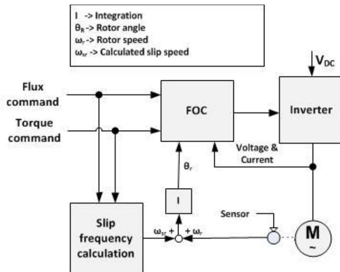
**Figure 93: Block diagram of indirect field-oriented control (IFOC) (49)**
