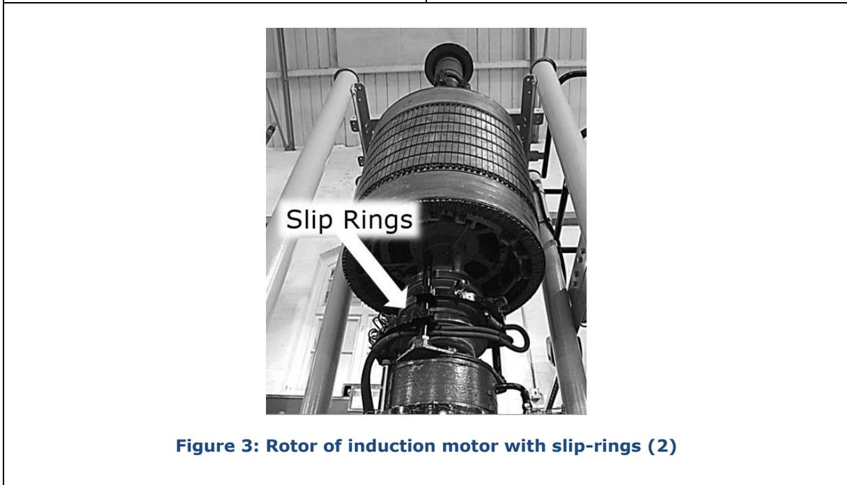
**Figure 3: Rotor of induction motor with slip-rings (2)**
