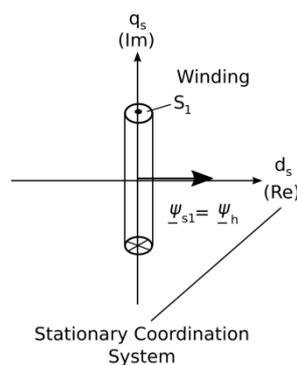
**Figure 81: Producing flux linkage with one winding (5)**
