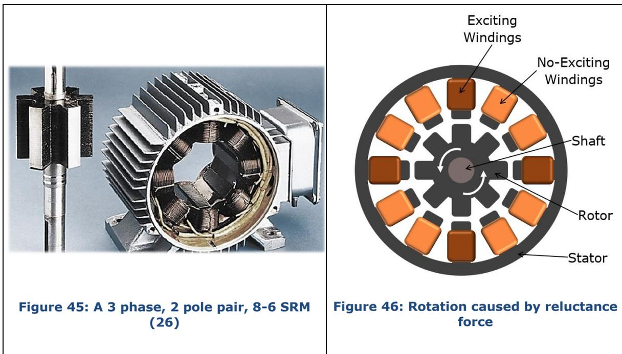
SRMs have a very simple structure as shown in Figure 45. Both the stator and the rotor have salient poles. There is no permanent magnet or other external excitation in a SRM. Concentrated windings are usually used for the stator. The relationship between the number of the stator teeth  $N_s$ , the magnetic pole pair number  $p$  and the number of the electrical phases  $N_{ph}$  for SRMs is written as:
