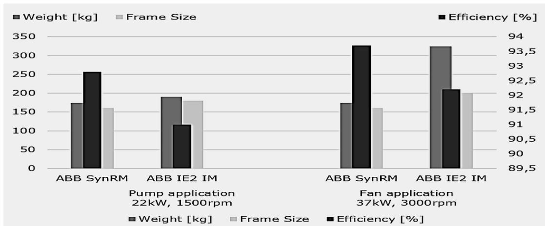
**Figure 26: Comparison of efficiency and power density aspects for synchronous reluctance vs. induction machines (data originating from ABB (17))**
