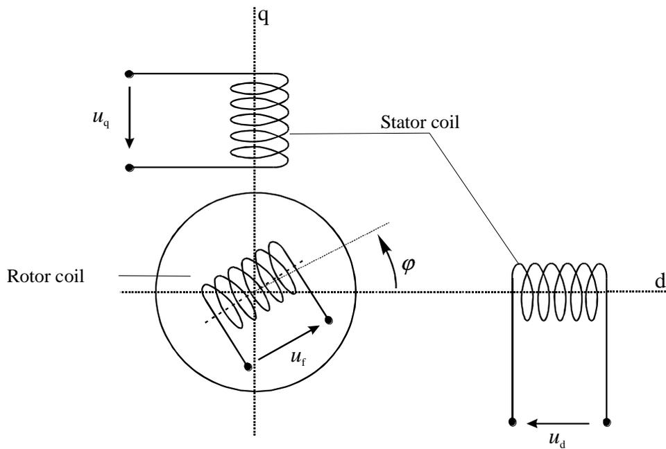
**Figure 87: Resolver for absolute position measurement (5)**
