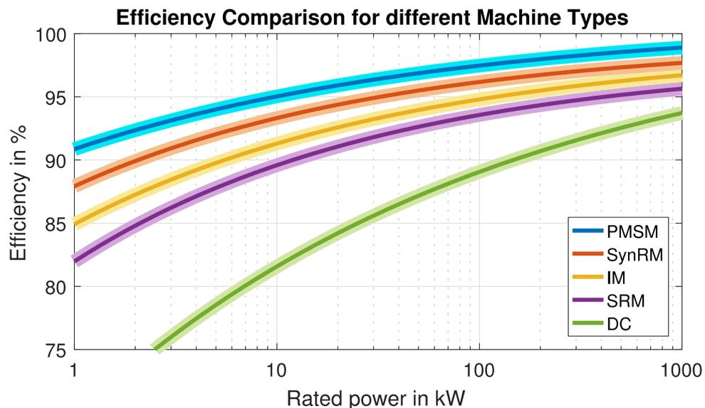
**Figure 100: Example comparison of efficiency for different machines (60), (61)**
