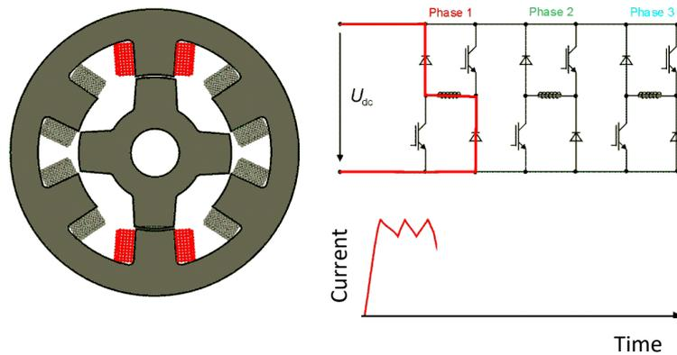
**Figure 53: Current flow of the de-magnetization state (5)**
