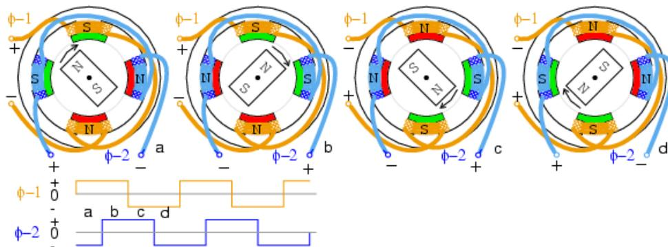
**Figure 67: Simplified permanent magnet stepper in full-step drive (31)**
