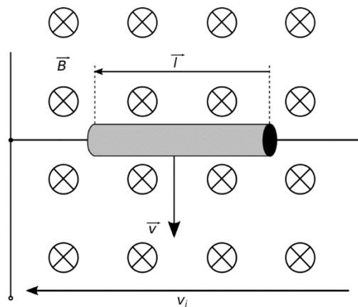
**Figure 83: Generation of an induced voltage (5)**
