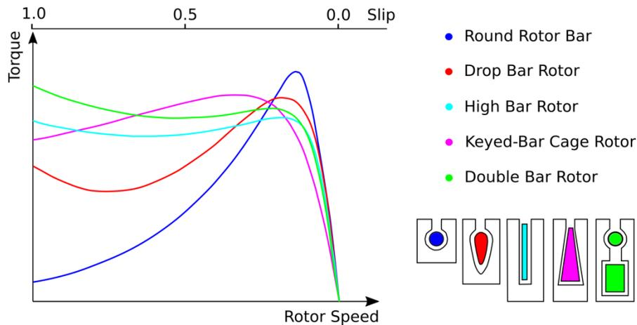
**Figure 8: Influence of the shape of rotor bars (5), (6)**
