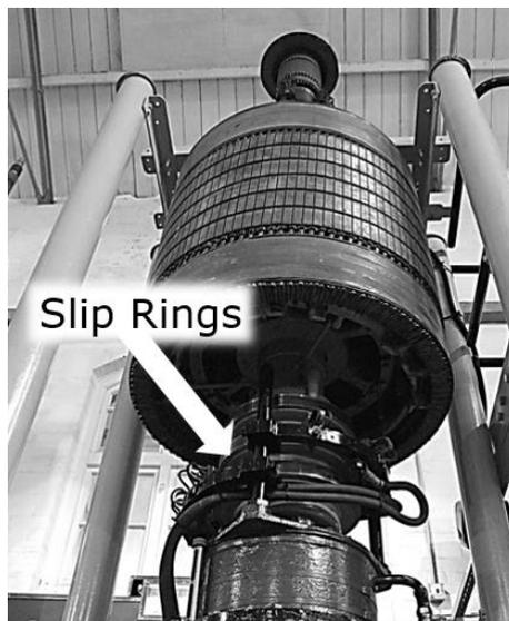
**Figure 3: Rotor of induction motor with slip-rings (2)**
