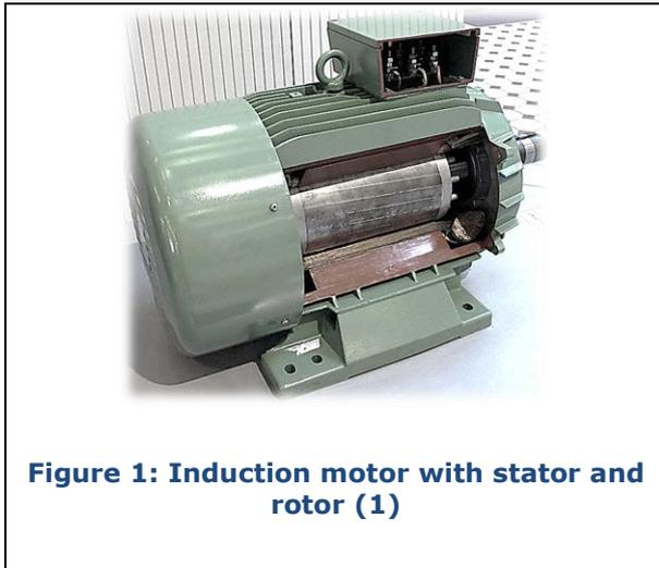
**Figure 1: Induction motor with stator and rotor (1)**
