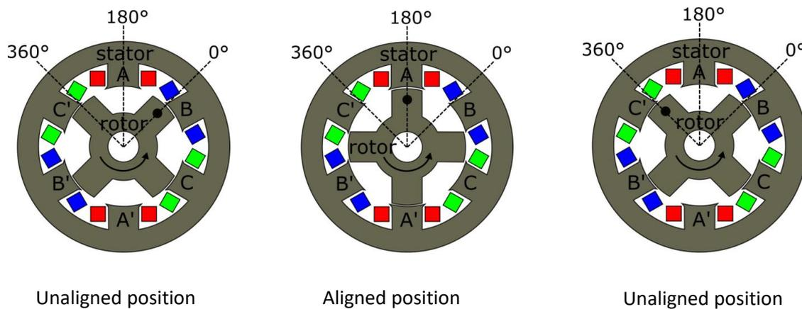
**Figure 54: Electrical cycle for phase "A" (7; 5)**
