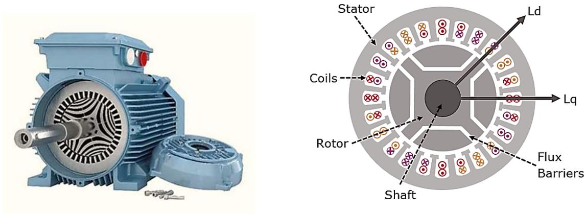
**Figure 24: Cross section of a synchronous reluctance machine by ABB (15) (left), and a schematic cross section (right)**
