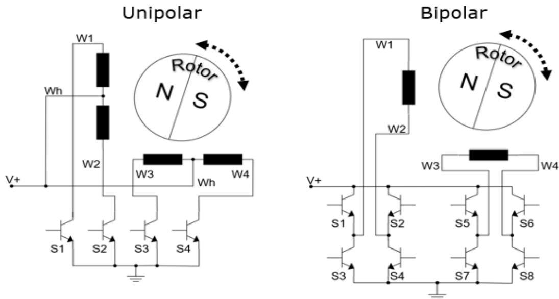
**Figure 73: Switches for bipolar and unipolar motor (36)**
