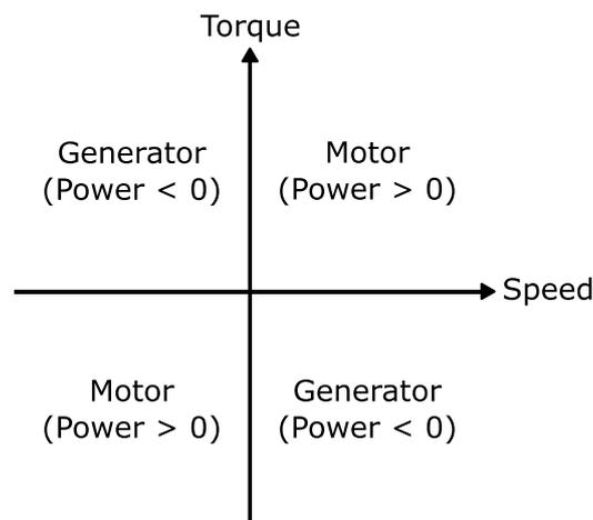
**Figure 76: Operation quadrants of electrical drives (5)**
