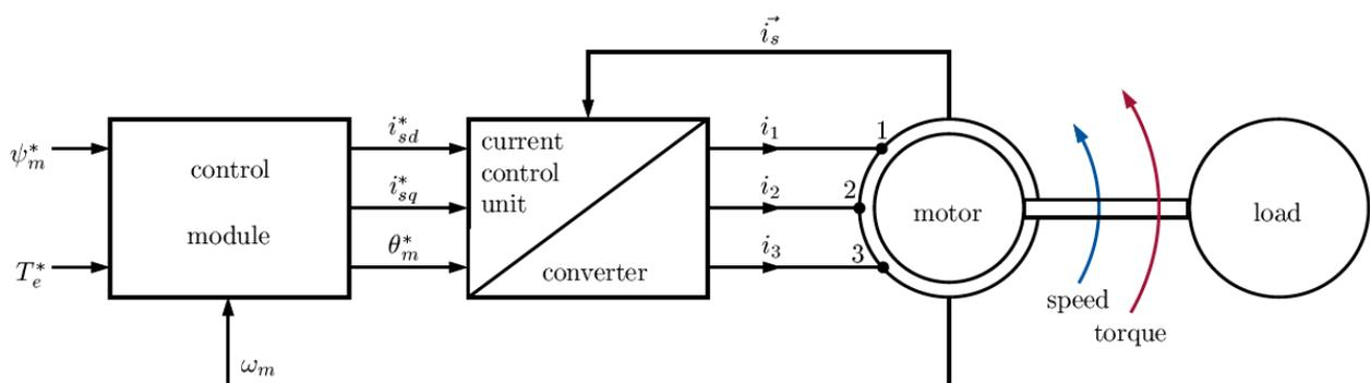
**Figure 12: Field-oriented control drive structure (5) (7)**
