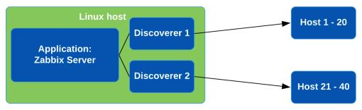
Figure 10.21 – Zabbix server multiple process setup diagram
