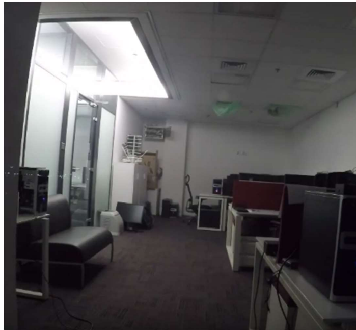
Figure 1. Example of the attack. A leaking HDD LED (the red LED at the center of the image) as captured by a hidden video camera eight meters away from the transmitting computer.
