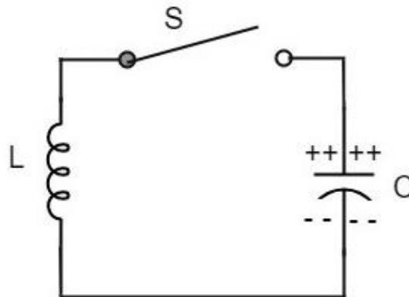
When the switch **S** is closed, the capacitor discharges and the current flows through the inductor. Due to the inductive effect, the current builds up slowly towards a maximum value. Once the capacitor discharges completely, the magnetic field around the coil is maximum.
