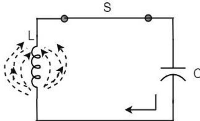
Now, let us move on to the next stage. Once the capacitor is discharged completely, the magnetic field begins to collapse and produces a counter EMF according to Lenz's law. The capacitor is now charged with positive charge on the upper plate and negative charge on the lower plate.
