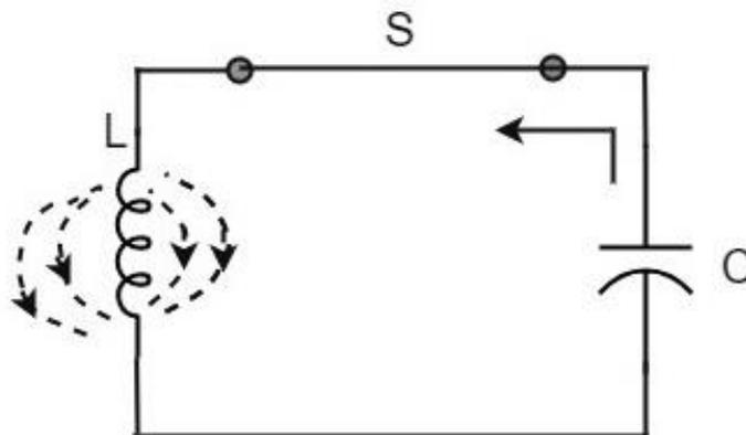
This continuation of charging and discharging results in alternating motion of electrons or an **oscillatory current**. The interchange of energy between L and C produce continuous **oscillations**.
