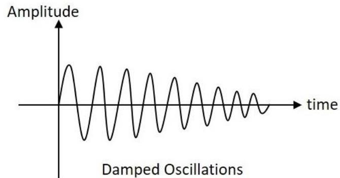
Damped oscillations are generally produced by the oscillatory circuits that produce power losses and doesn't compensate if required.
