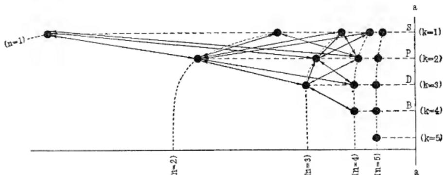
Diagram of the series spectrum of sodium.
