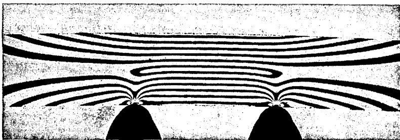
FIGURE 27J Photoelastic effect in a plastic beam loaded at two points. (Courtesy of R. W. Clough, Jr.)
