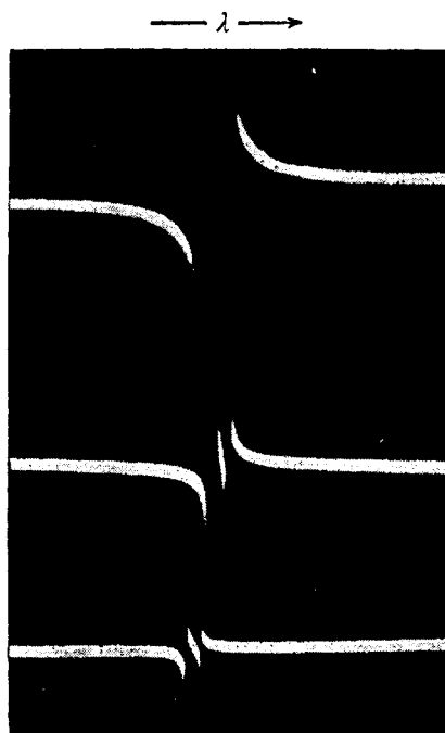
FIGURE 23F Anomalous dispersion of sodium vapor at three different gas densities. ( Courtesy of Cario. )
