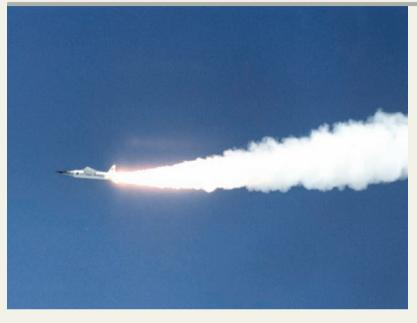
Chemical reactions initiated in the Pegasus rocket accelerate NASA's X-43A aircraft to hypersonic speeds. In a November 2004 test flight, the X-43A approached Mach 10, ten times the speed of sound. *NASA Dryden Flight Research Center*
