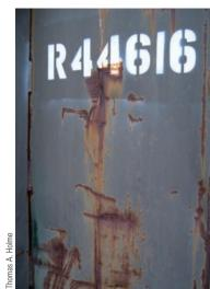
**Figure 13.22** The photo shows corrosion at scratches on a dumpster. In designs for large metal objects subject to rough handling, corrosion prevention is usually only partially successful.
