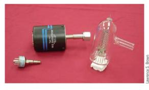
The photo shows (from left to right) a thermocouple gauge, a capacitance manometer, and an ionization gauge. The electronics needed to operate the gauges are not shown.
