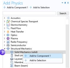
When adding additional physics, you need to make sure that materials included in the **Materials** node have all of the required properties for the selected physics. In this example, all properties are already available for copper and titanium.
