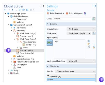
2 Click the **Build Selected** button not to create the cylindrical part of the titanium bolt that runs through the busbar.
