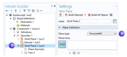
4 In the **Graphics** window, click face 8, as shown in the figure below, to add it to the **Planar face** list in the Settings window for **Work Plane**.
