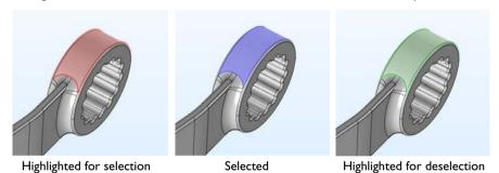
To select internal surfaces that are hidden behind the one closest to you, use one of the following methods to cycle through the boundaries at the mouse pointer: roll the mouse scroll wheel, use the keyboard + and - buttons, use the keyboard arrow-up and arrow-down buttons, or use two-finger drag on a touchpad.
