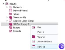
3 In the Settings window for Surface, click the Replace Expression button and select Model > Component I > Solid Mechanics > Stress > solid.mises-von Mises stress - N/m² by double-clicking. When you know the variable name beforehand, you can also directly enter solid.mises in the Expression field. Now edit this expression to: solid.mises>200[MPa].
