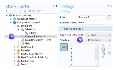
This creates an operator called aveop1. This operator is now available to calculate the average of any quantity defined on the selected domains. Later, we use this tool to calculate the average temperature, but it can also be used to calculate average electric potential, current density, and so forth.
