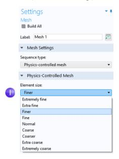
2 Click the **Build All** button in the **Settings** window or on the **Mesh** toolbar. The resulting mesh will require about 5GB to solve. If you have a computer with less than 5GB of RAM you can select **Fine** from the **Element size** list (instead of **Finer**.)
