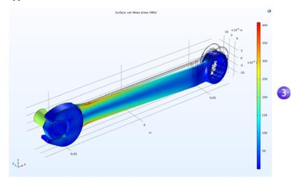
For a typical steel used for tools like a wrench, the yield stress is about 600 MPa, which means that we are getting close to plastic deformation for our 150 N load (which corresponds to about 34 pounds force). You may also be interested in a safety margin of, say, a factor of three. To quickly assess which parts of the wrench are at risk of plastic deformation, you can plot an inequality expression such as solid.mises>200[MPa].
