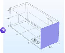
In the **Model Builder**, right-click **Heat Transfer in Solids ...** At the boundary level, select **Flow Conditions>Outflow**. An **Outflow** node **...** is added to the model tree.
