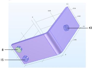
4 In the Settings window for Heat Flux under Heat Flux, click the Convective heat flux button. Enter htc in the Heat transfer coefficient field, h.
