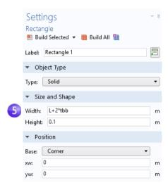
6 Create a second rectangle. Under Work Plane I, right-click Plane Geometry ⋈ and select Rectangle □. Under Size, enter:
