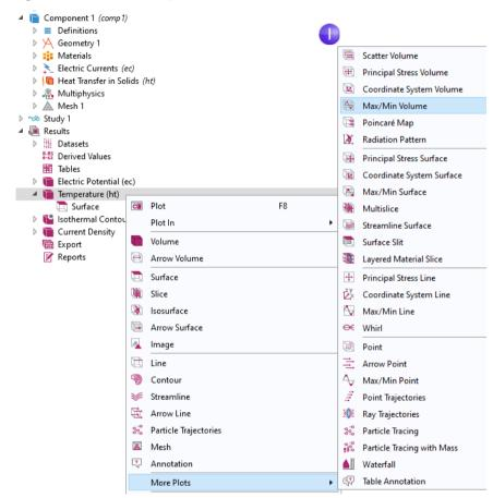
2 In the Settings window for Max/Min Volume under Expression, click the Replace Expression button ►. Go to Model > Component I > Heat Transfer in Solids > Temperature > T - Temperature - K and double-click or press Enter to select. You
