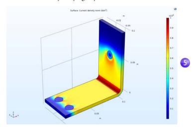
6 Click and drag the busbar in the **Graphics** window to view the back. Continue rotating the image to see the high current density around the contact surfaces of each of the bolts.
