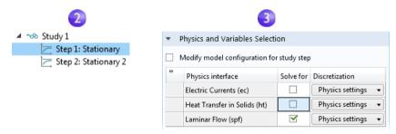
3 In the Settings window for Stationary, locate the Physics and Variables Selection section. In both the Electric Currents (ec) and the Heat Transfer in Solids (ht) rows, click to change the check mark ☐ to an ☐ in the Solve for column, removing the Joule heating effect from Step 1.
