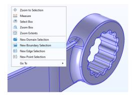
Click to select the boundaries to which you would like to apply the boundary condition. (In this case, the top socket face; boundary III.) Then, right-click again and select **Boundary Load**, as shown in the figure below.
