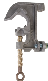
T6000658 Aluminum body, Smooth jaws, Bronze eyescrew with Acme threads, Drilled for 5/8-11 UNC threaded ferrule
