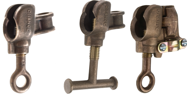
Clamp C6002100 Drilled for 5/8-11 UNC threaded ferrule or Clamp C6002101 Tapped for 5/8-11 UNC threaded ferrule Clamp T6002320 Tapped for 5/8-11 UNC threaded ferrule for threaded stud ferrule on #2 to 4/0 grounding cable Clamp C6002300 with pressure terminal for plain-plug ferrule on #2 to 4/0 grounding cable
