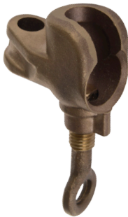
Ball Stud Ground Clamp accepts 30 mm Ball Studs Grade 5H Rated Catalog No. PSC6003494 Drilled for 5/8-11 UNC threaded ferrule
