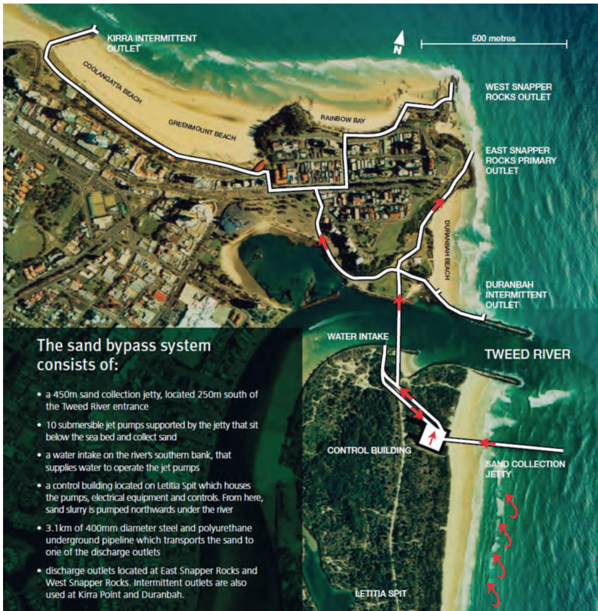
Figure 41. Tweed River Sand Bypassing System. (SOURCE: TWEED RIVER ENTRANCE SAND BYPASSING PROJECT WWW.TWEEDSANDBYPASS.NSW.GOV.AU)
