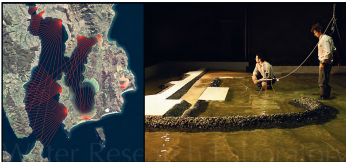
Figure 7. Examples of wave penetration numerical and physical models.
