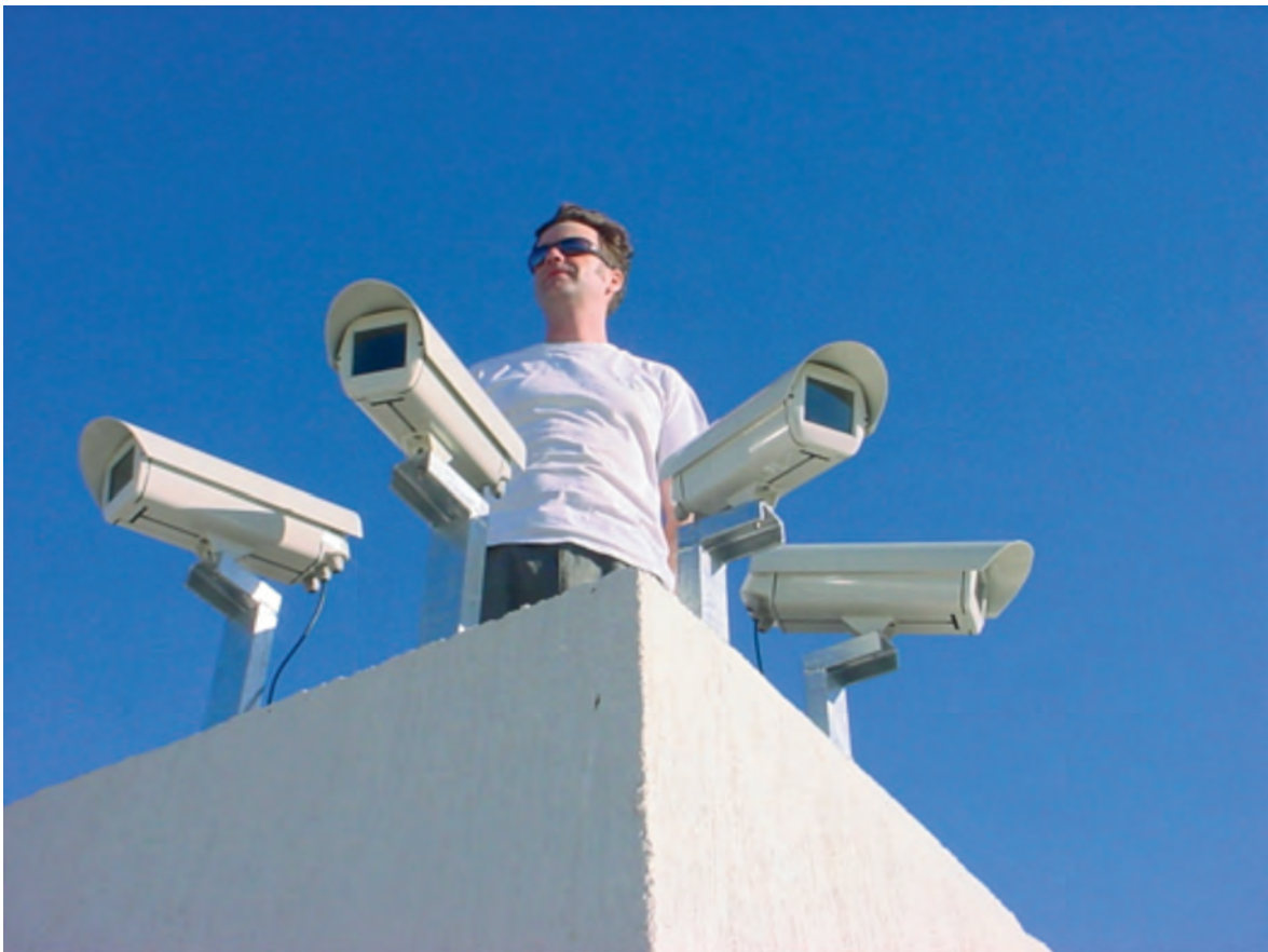
Figure 6. Argus system for monitoring beach movements and breaking waves.
